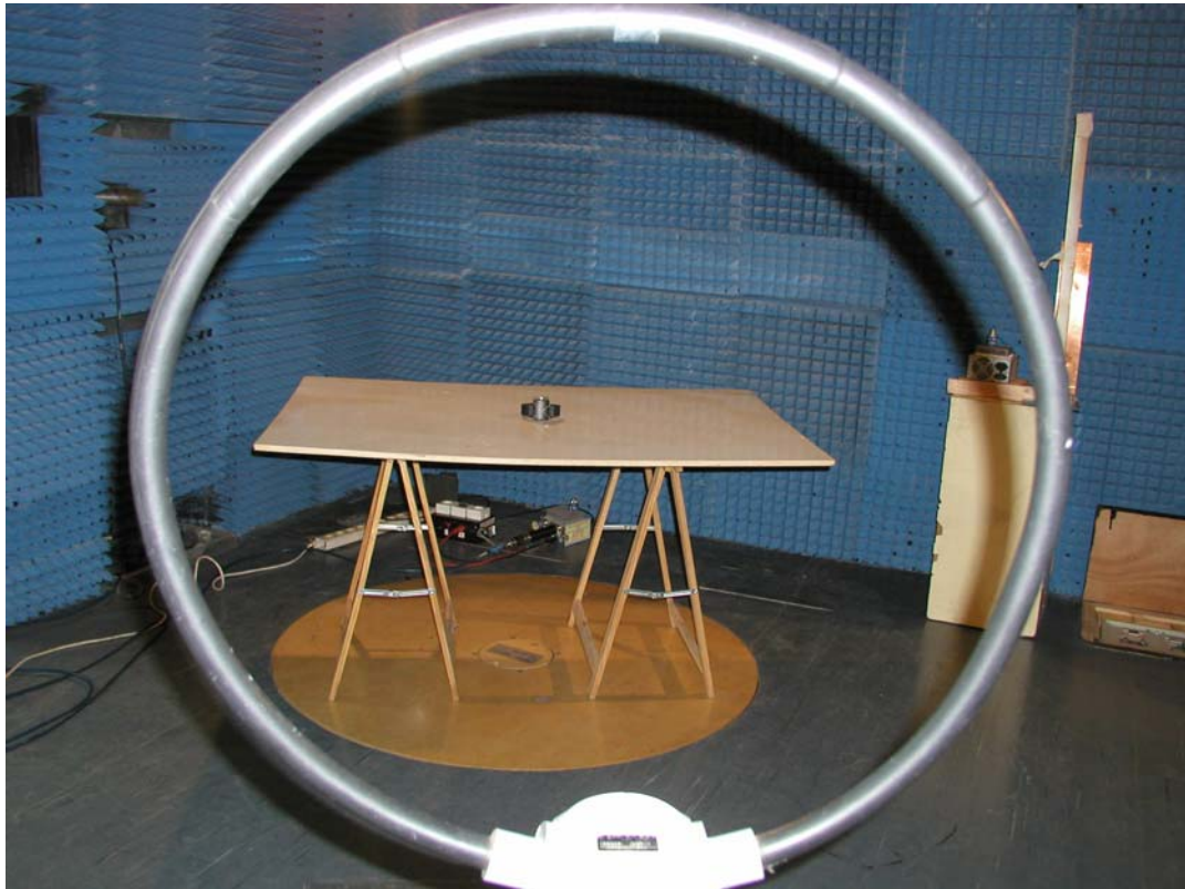
Photograph/ 1 Radiated Emission Test Setup up to 30MHz
