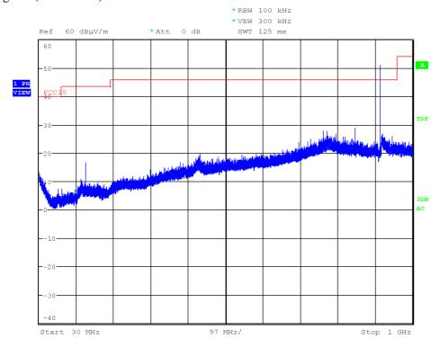
Note: The carrier was attenuated using a Notch filter. The peak above the limit is the carrier frequency.
