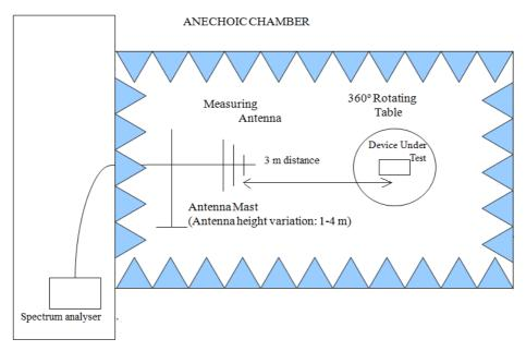
Shielded Control Room For Radiated Measurements
