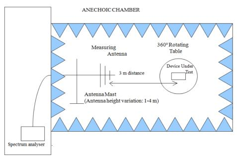
Shielded Control Room For Radiated Measurements
