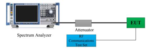
Note: The Insertion loss of the RF cable, Attenuators was offset into the Spectrum Analyzer.
