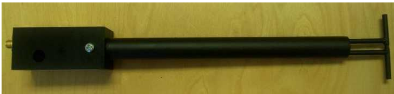
Figure 1 – MVG COMOSAR Validation Dipole
