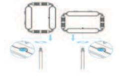
To attach a smartphone device to the Video Voyager, place your smartphone into the included phone holder, ensuring it is securely in place. Once the smartphone is secure, screw the phone holder to the inner mounting screw.
