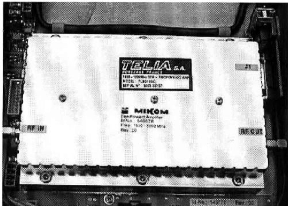
figure 2-9 Top view of the feed forward amplifier
