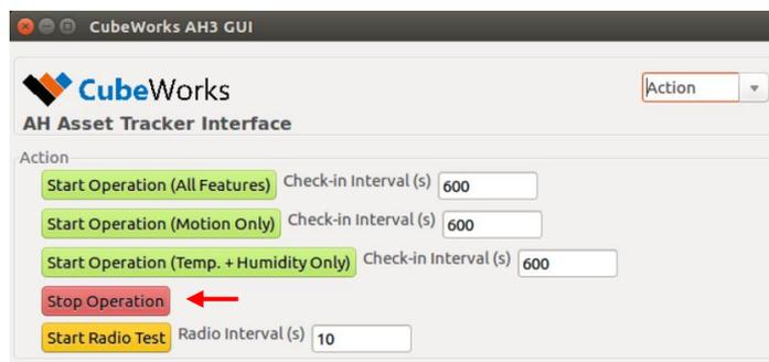
**Stopping AH100 Sensing Operation / Radio Test**
