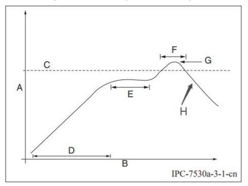
Set oven temperatures according to the following curve.
