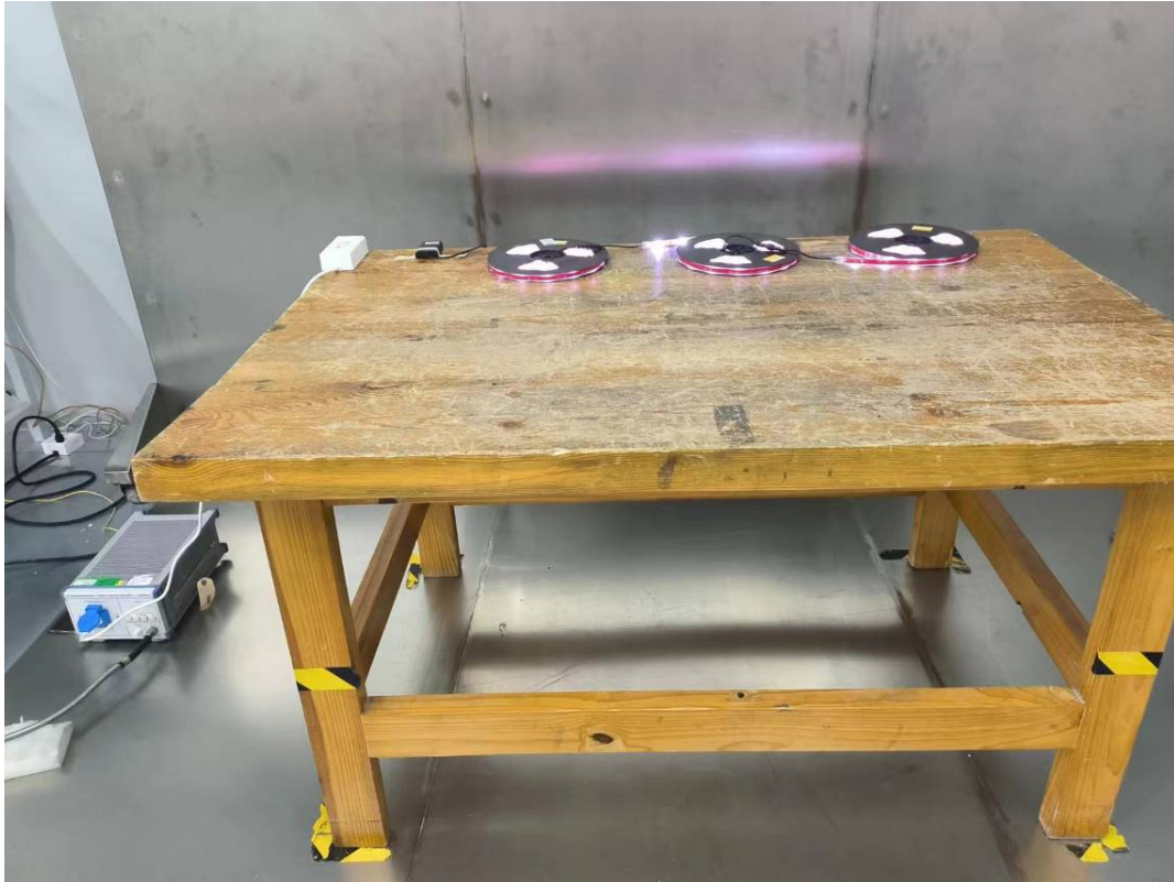
Conducted Emissions Side View–For Model H6176 (Adapter 1)
