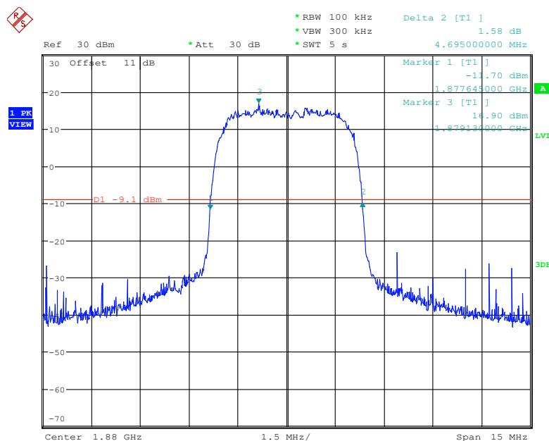
**26 dB Emissions for HSDPA (16QAM) Mode, High channel**
