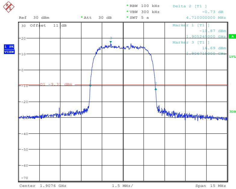
**99% Occupied Bandwidth for GSM (GMSK) Mode, Low channel**
