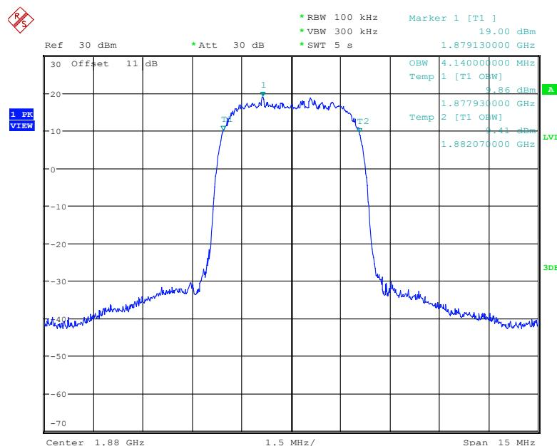
**99% Occupied Bandwidth for RMC (BPSK) Mode, High channel**
