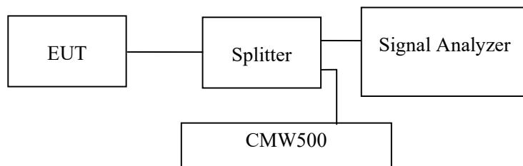
Note: the path loss (cable loss and attenuator) has included in the result.
