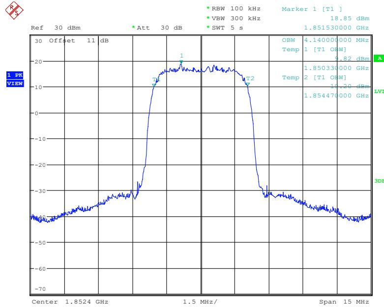
**99% Occupied Bandwidth for RMC (BPSK) Mode, Middle channel**
