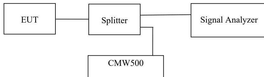
Note: the path loss (cable loss and attenuator) has included in the result.
