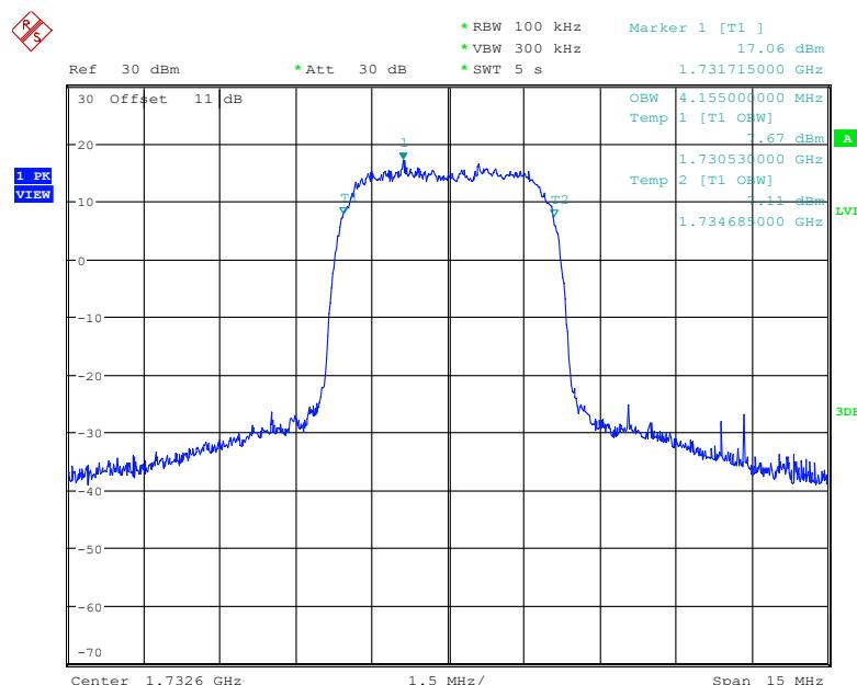
**99% Occupied Bandwidth for HSDPA (16QAM) Mode, High channel**
