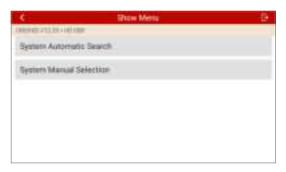
Tap "System Automatic Search" to scan which systems are equipped on the test vehicle automatically.
