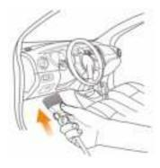
b) For non-standard OBD II DLC, connect one end of the adaptor to the diagnostic cable, and the other end to the vehicle's DLC port.
