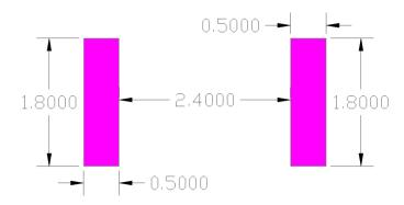
◆ 2<sup>nd</sup> Layout Dimensions in Clearance area(size=8.0\*3.0mm)
