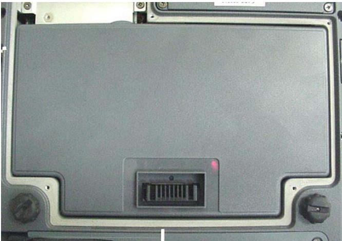
Internal Li-ion Battery 11.1 V, 3600 mAh (Model: T8M-E)
