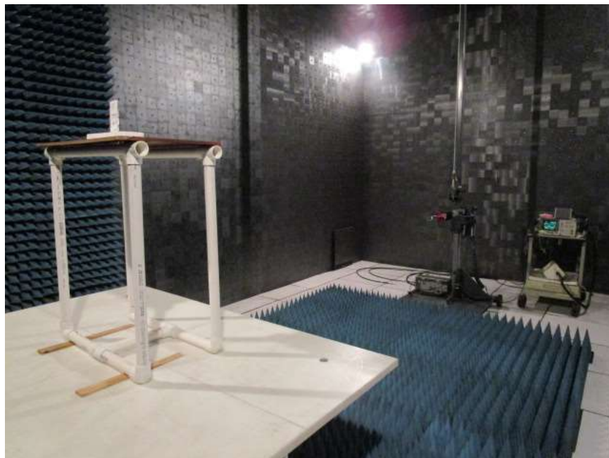
Radiated Emissions Test Setup 18 to 26 GHz
