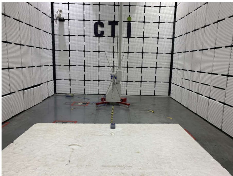
Radiated spurious emission Test Setup-1(Below 1GHz)
