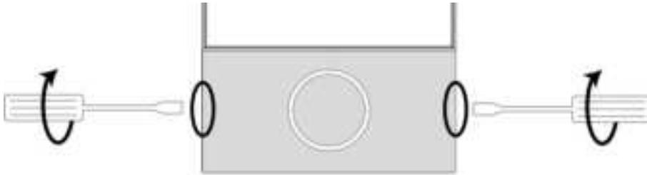
**Figure 3.9** - Opening the housing - Step 1
