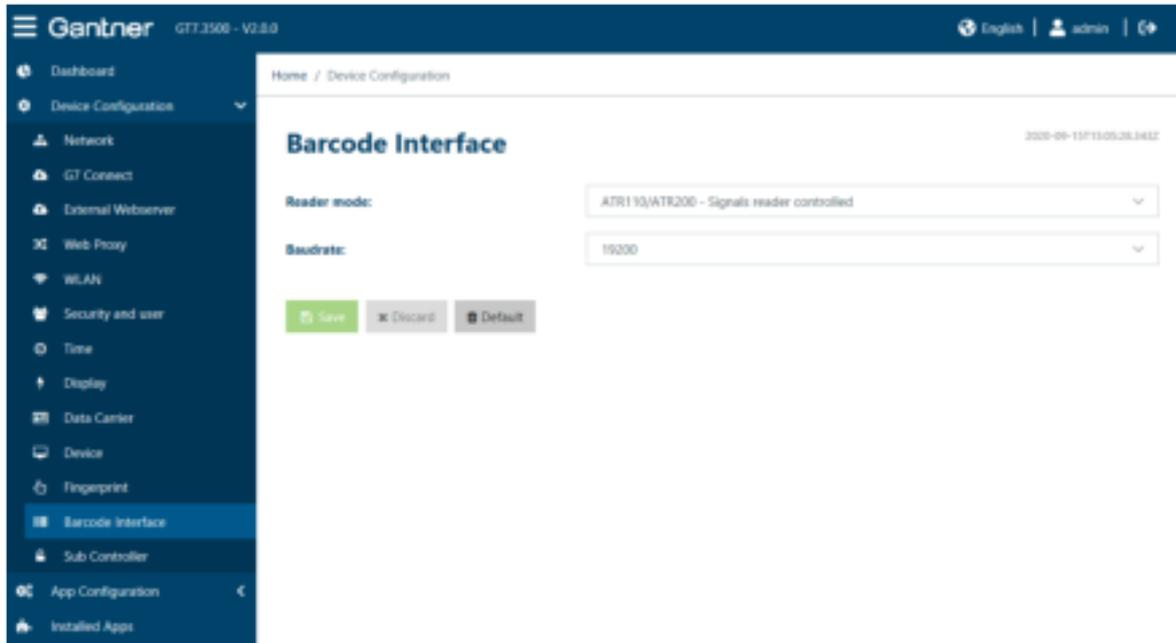
**Figure 5.34** – GT7 terminal web interface – Barcode Interface
