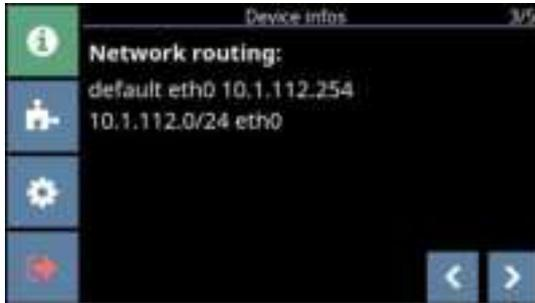
**Figure 5.6** - Device Information - Page 3, Network routing
