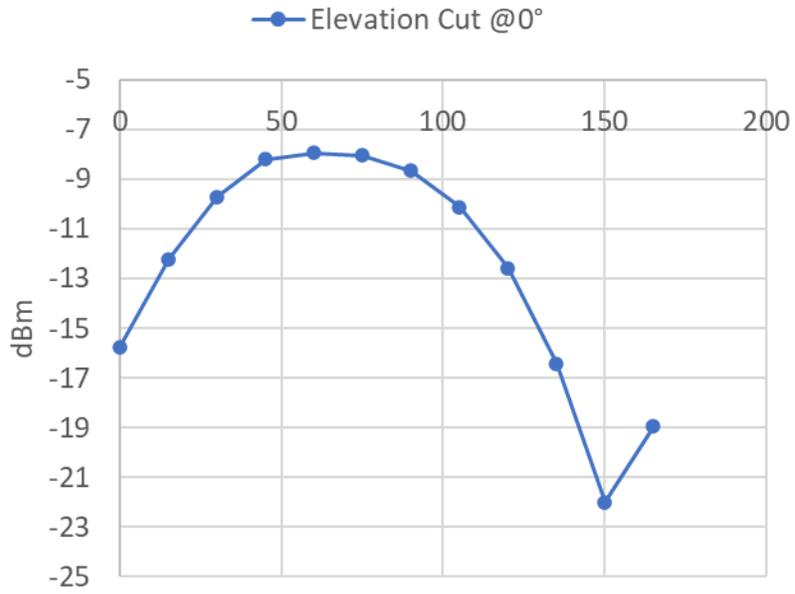
**Figure 2a** Left Hearing Aid Elevation cut @ 0 degrees from X axis.
