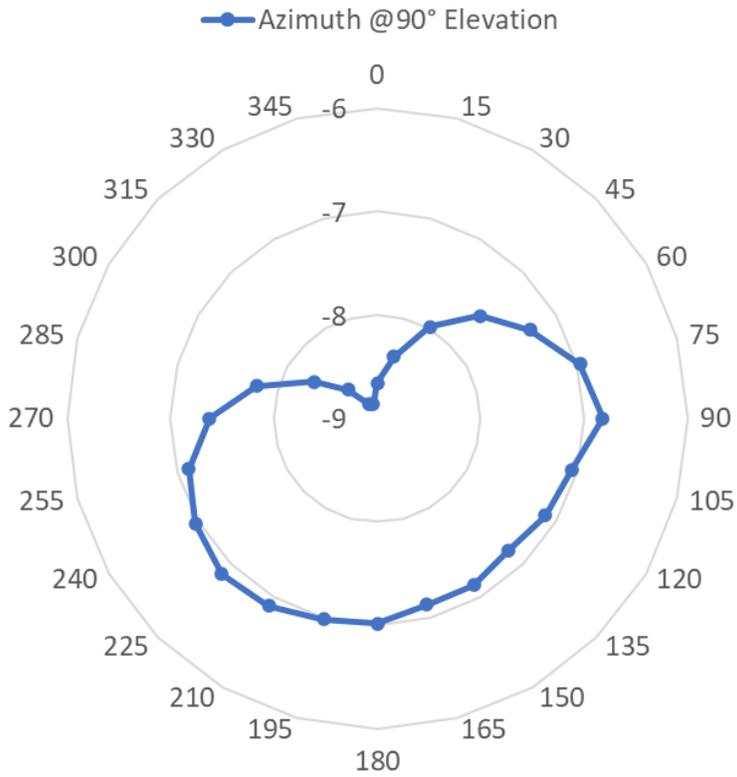
**Figure 2b** Left Hearing Aid Antenna Azimuth Cut @ 90 degrees from Z axis.
