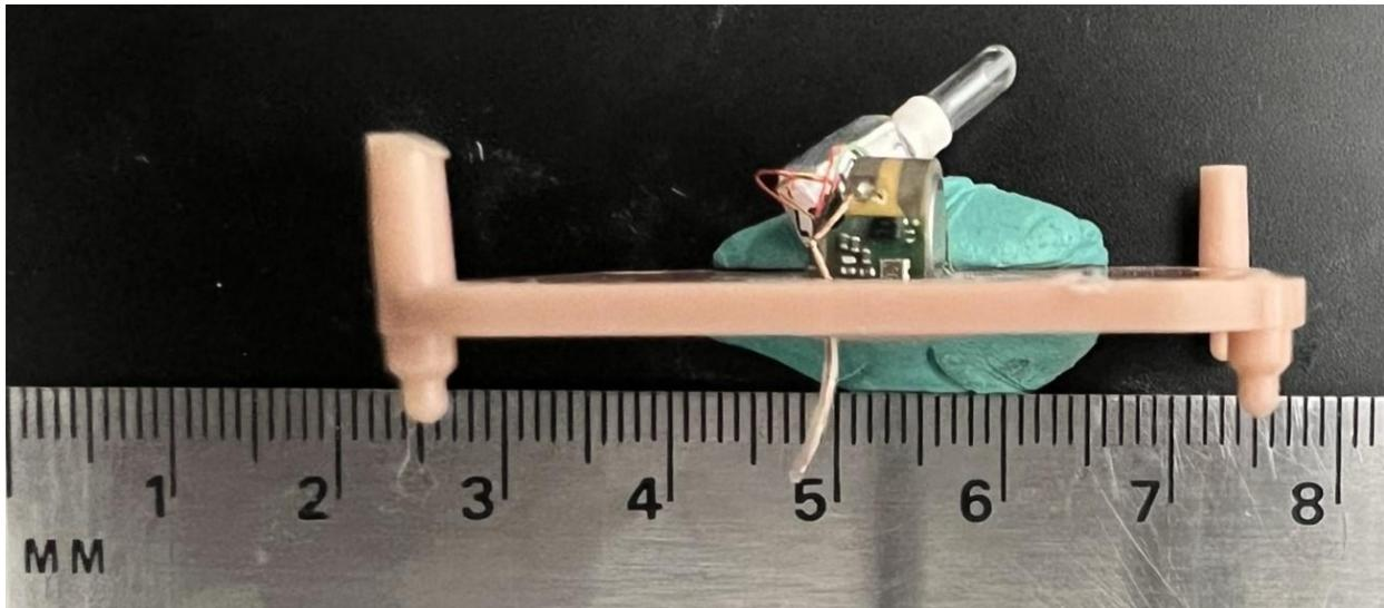
**Figure 1** 2.4 GHz Antenna (scale in mm)
