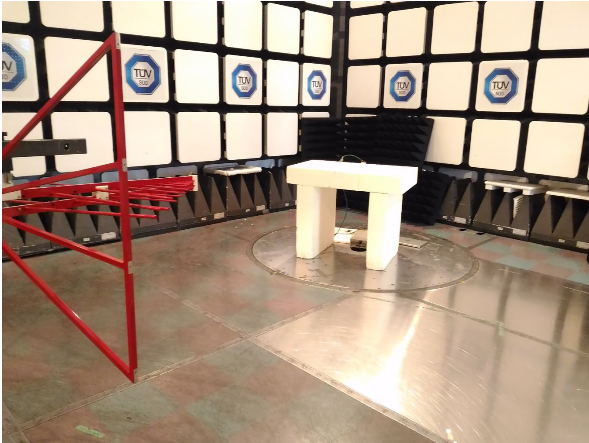
Figure 10 – Radiated Emissions Setup 30 MHz to 1 GHz
