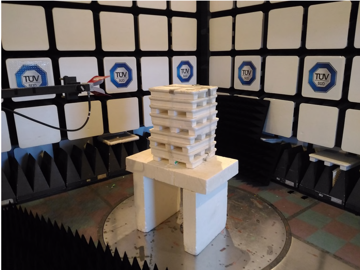
Figure 5 – Radiated Emissions Setup 10 GHz to 18 GHz
