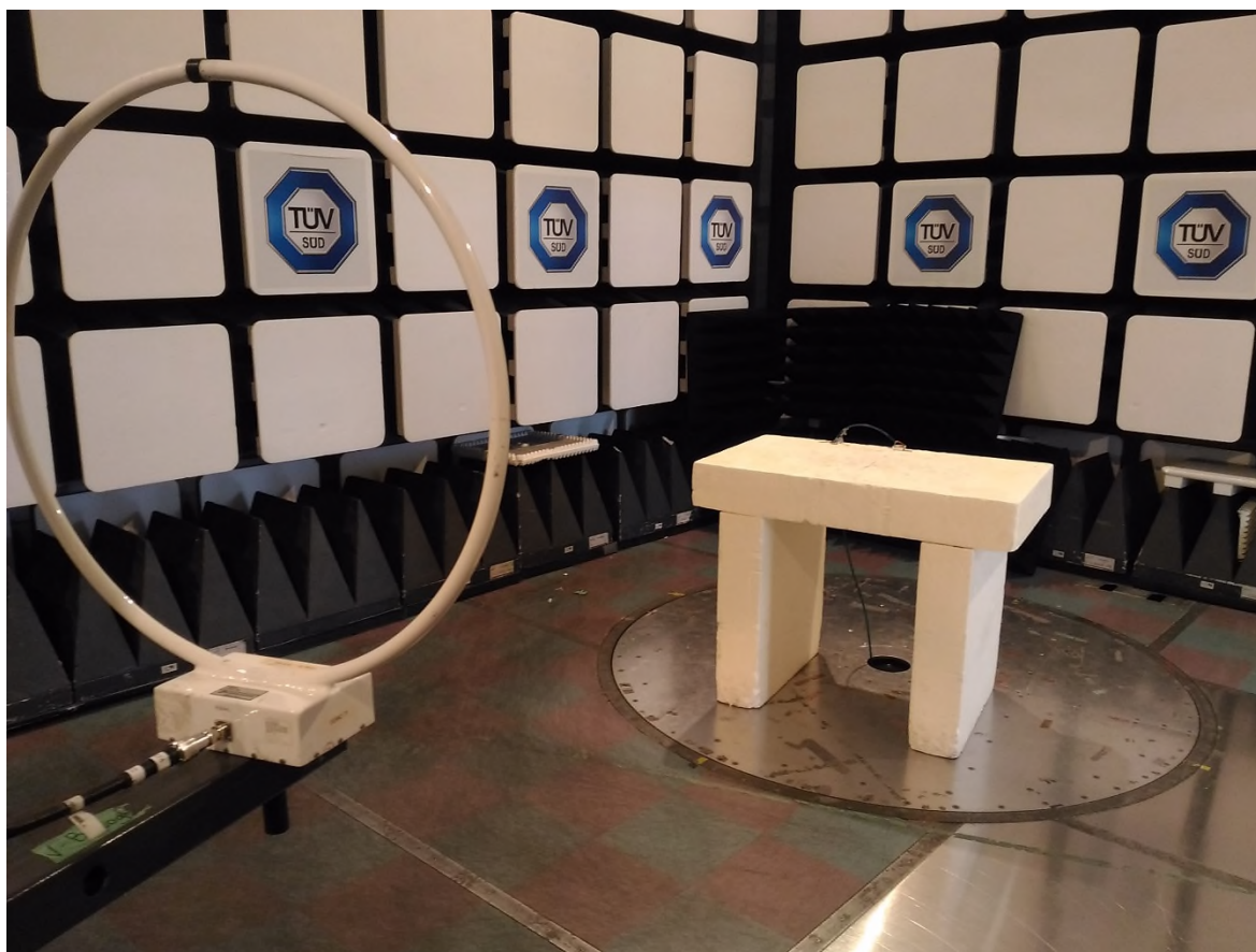
Figure 9 – Radiated Emissions Setup 9 kHz to 30 MHz
