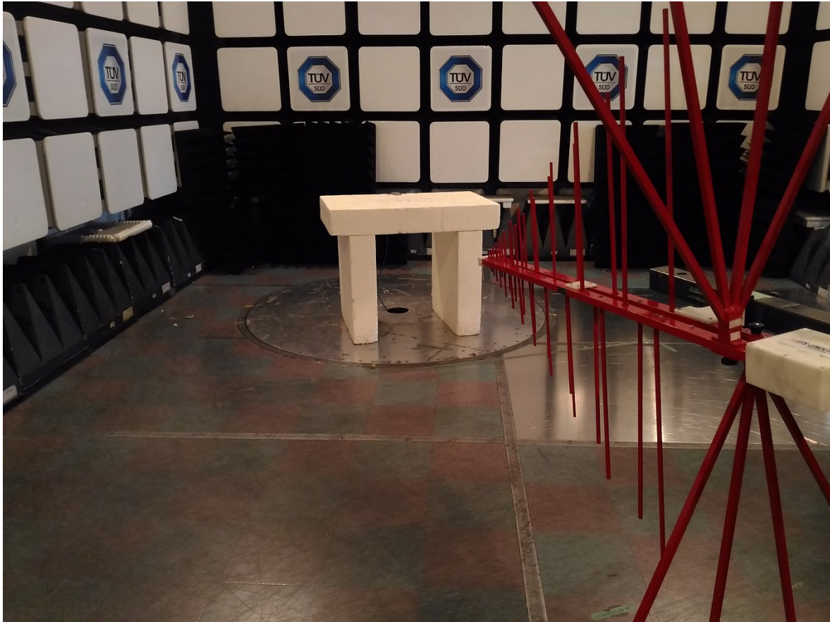
Figure 3 – Radiated Emissions Setup 30 MHz to 1 GHz
