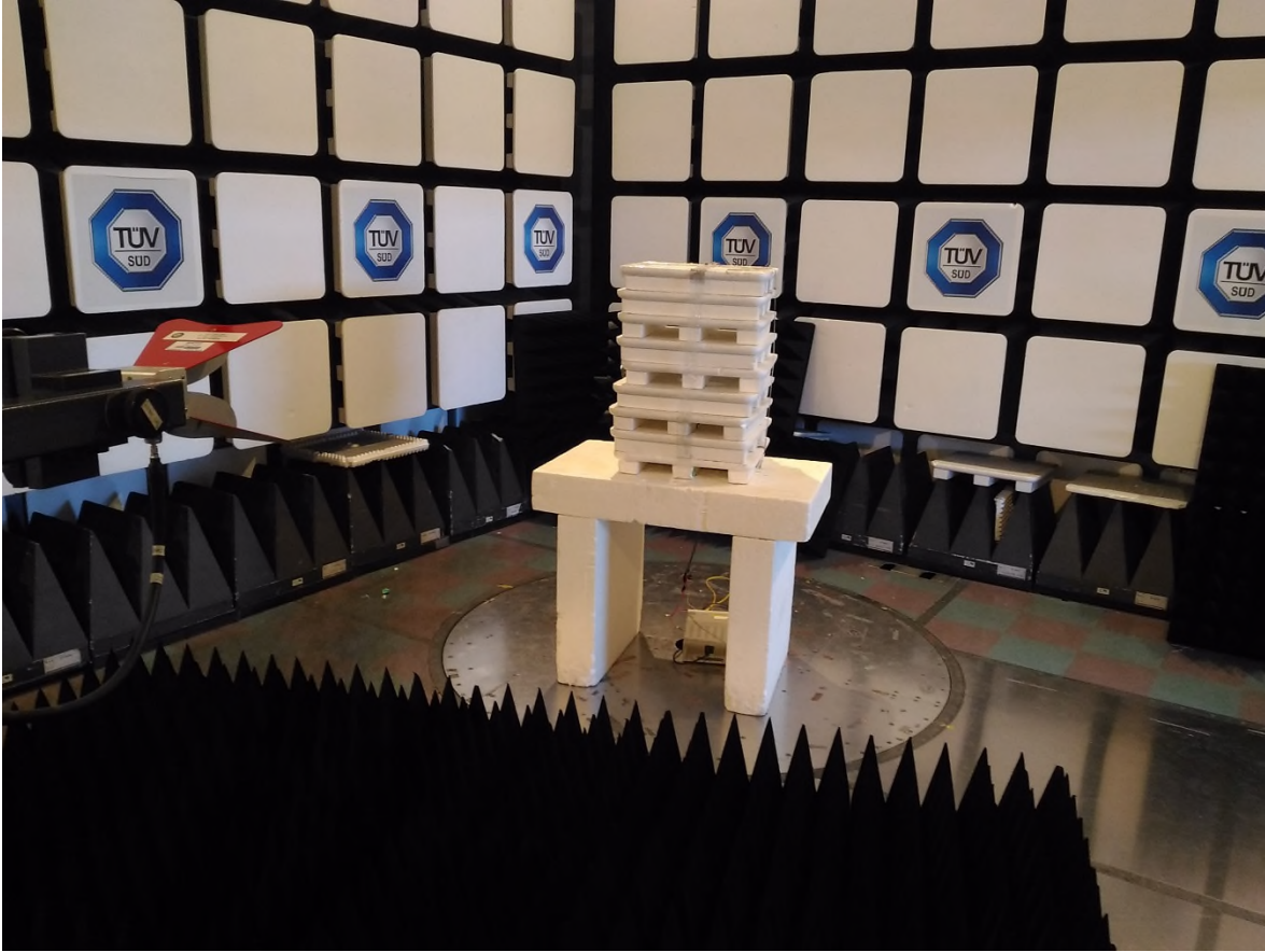
Figure 4 – Radiated Emissions Setup 1 GHz to 10 GHz
