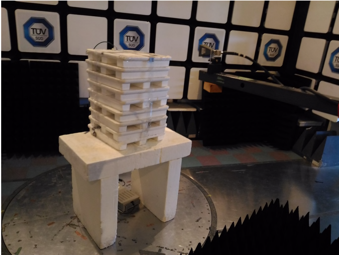
Figure 13 – Radiated Emissions Setup 18 GHz to 25 GHz
