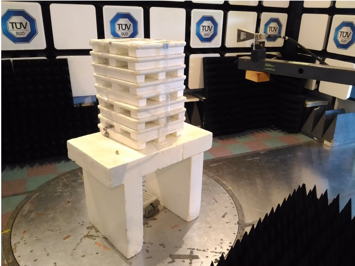
Figure 6 – Radiated Emissions Setup 18 GHz to 25 GHz
