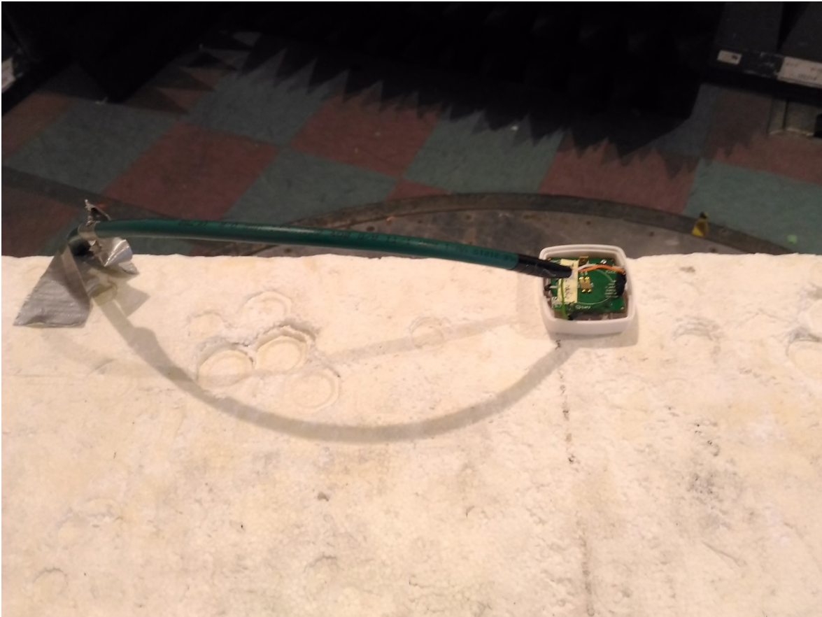
Figure 8 – Radiated Emissions Setup EUT setup for max emissions
