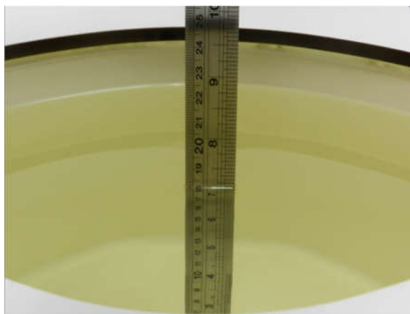
Fig 11.1 Photo of Liquid Height for Body SAR
