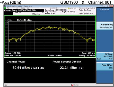
$PAPR (dB) = P_{Pk} (dBm) - P_{Avg} (dBm) = 30.67 dBm - 30.61 dBm = 0.06 dB$
