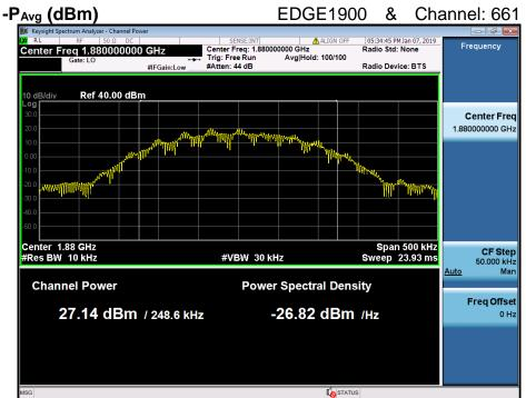
PAPR (dB) =  $P_{Pk}$  (dBm) -  $P_{Avg}$  (dBm) = 30.53 dBm - 27.14 dBm = 3.39 dB
