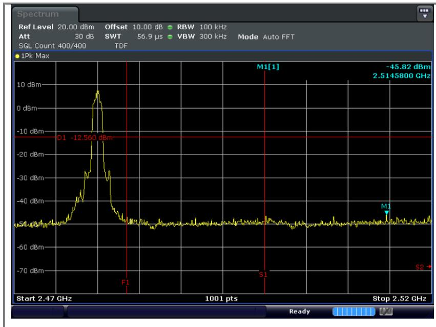
Unwanted Emission data (With Hopping Enabled)
