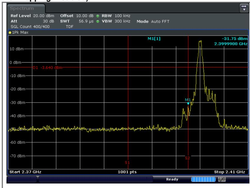
**Band-edge data (With Hopping Enabled)**
