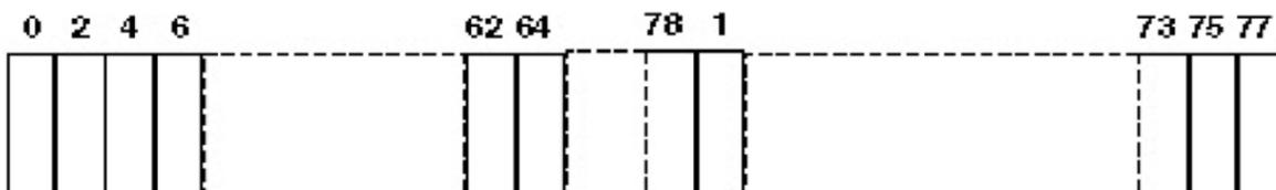
Each frequency used equally on the average by each transmitter. The system receiver have input bandwidths that match the hopping channel bandwidths of their corresponding transmitters and shift frequencies in synchronization with the transmitted signals.
