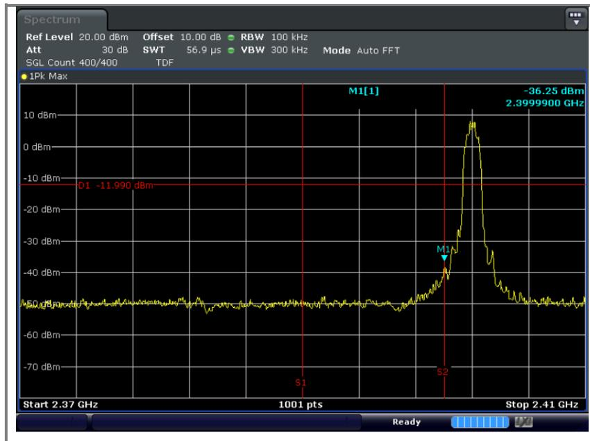
**Band-edge data (With Hopping Enabled)**
