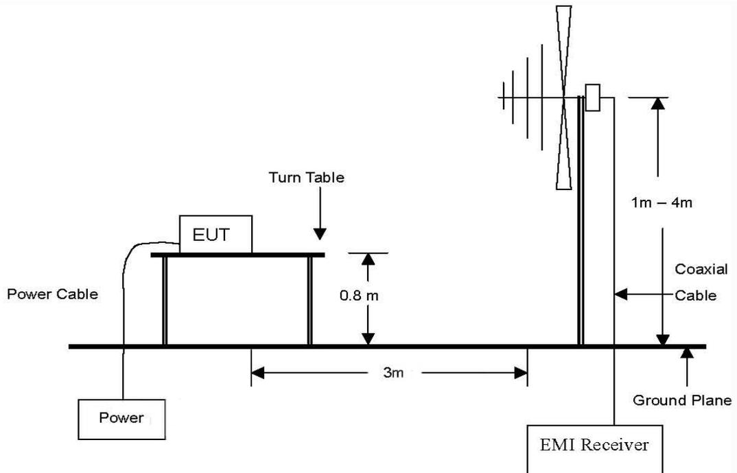
The diagram below shows the test setup that is utilized to make the measurements for emission Above 1 GHz emissions.
