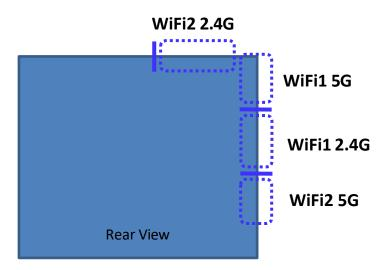
Antenna Type: WiFI 1(2.4G/5G): Metal Insert , WiFi2(2.4G): Metal Insert , WiFi2(5G): LDS The antennas can be seen in the internal photos.
