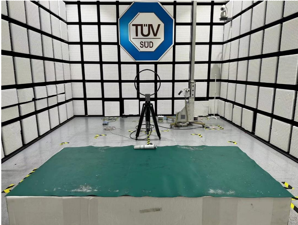
Radiated Emission Setup 9kHz ~ 30MHz
