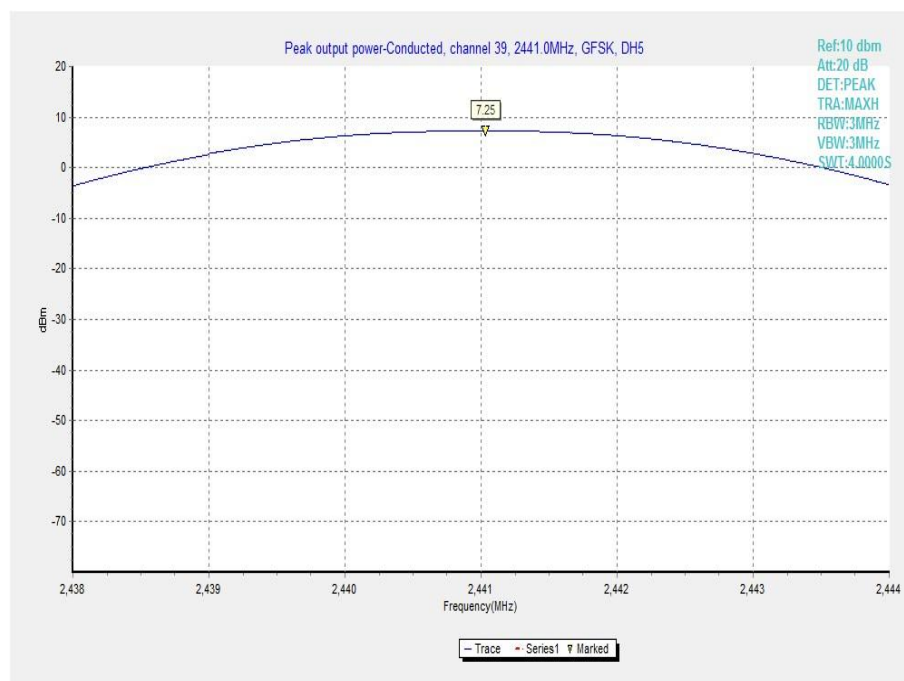
Fig. 2 Maximum Peak Output Power(GFSK, Ch 39)
