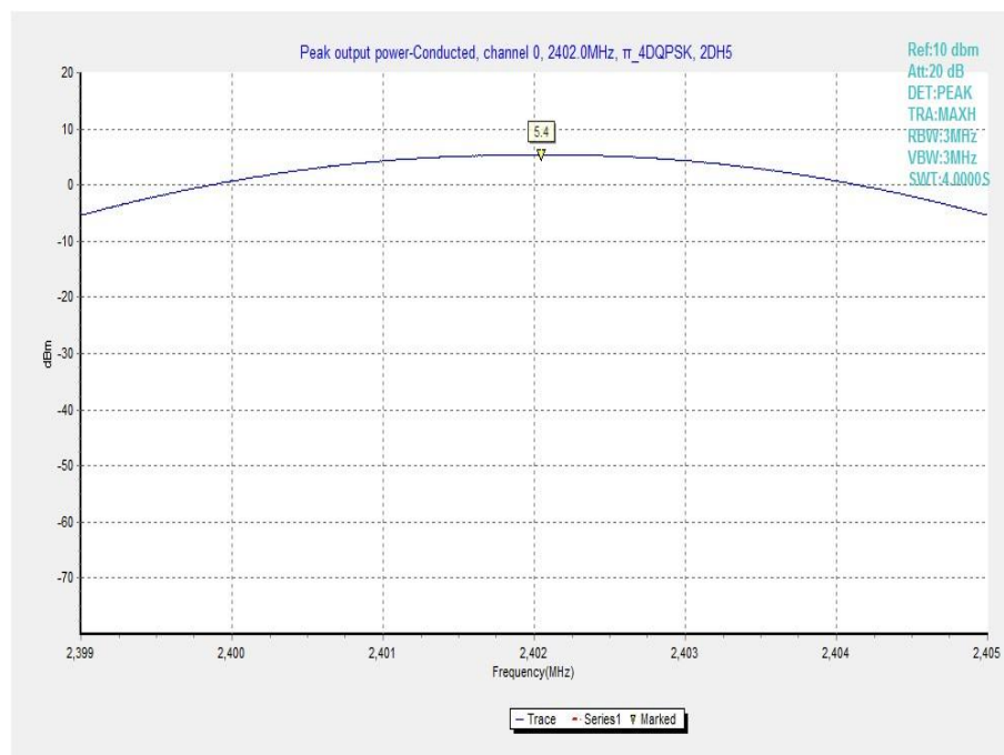
Fig. 4 Maximum Peak Output Power( \pi/4 DQPSK, Ch 0)
