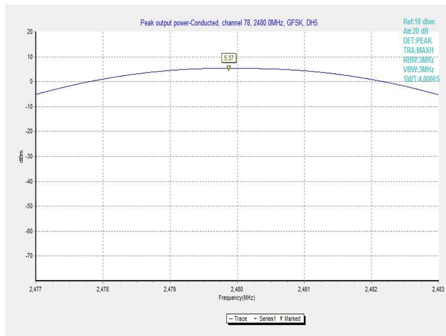
Fig. 3 Maximum Peak Output Power(GFSK, Ch 78)
