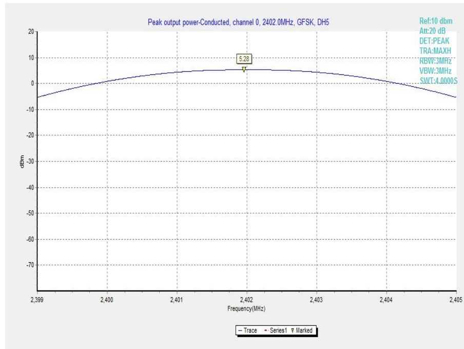
Fig. 1 Maximum Peak Output Power(GFSK, Ch 0)
