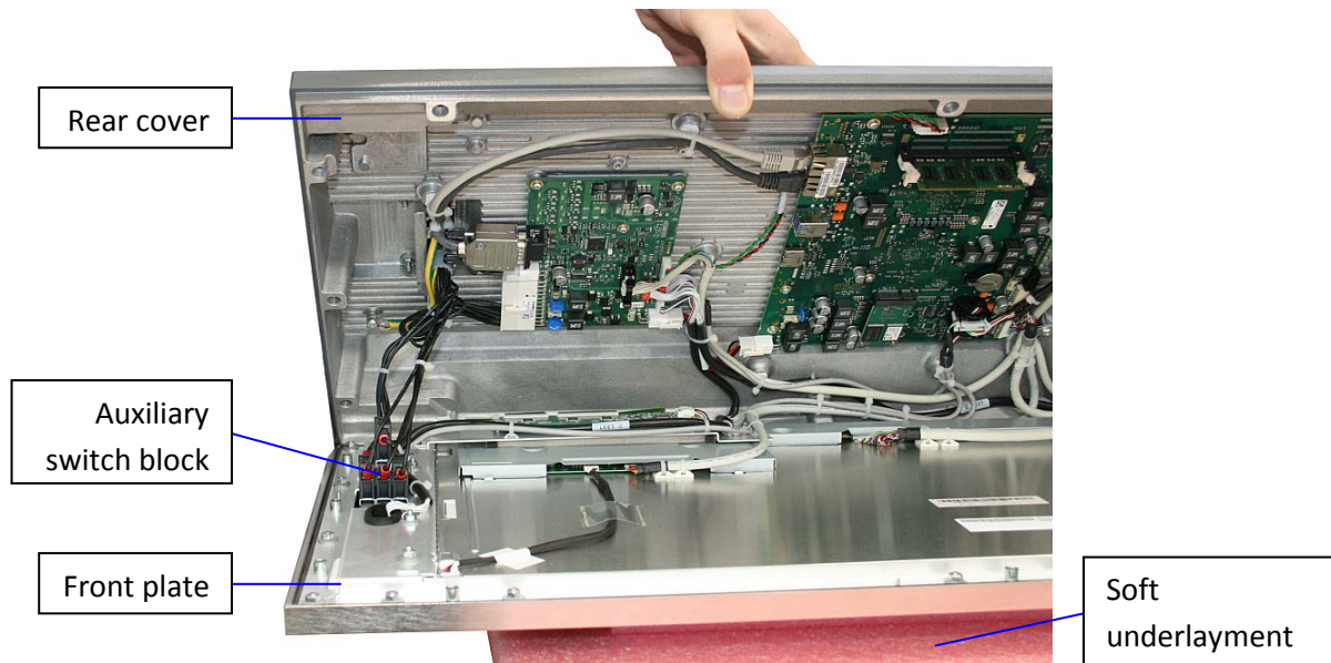
Fig. 26: Carefully open the CC300 a few inches
