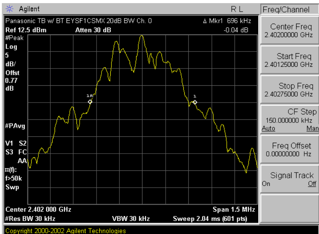
Plot 6-1. 20dB Bandwidth Plot (Bluetooth – Ch. 0)
