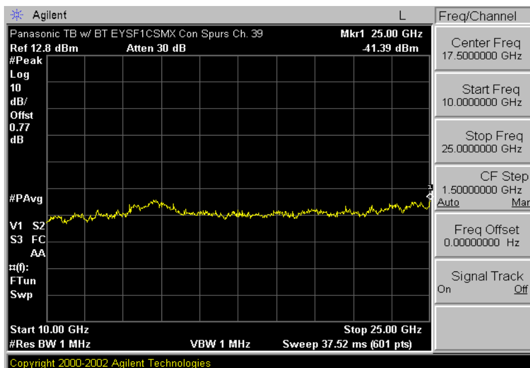
Plot 6-13. Conducted Spurious Plot (Bluetooth – Ch. 39)
