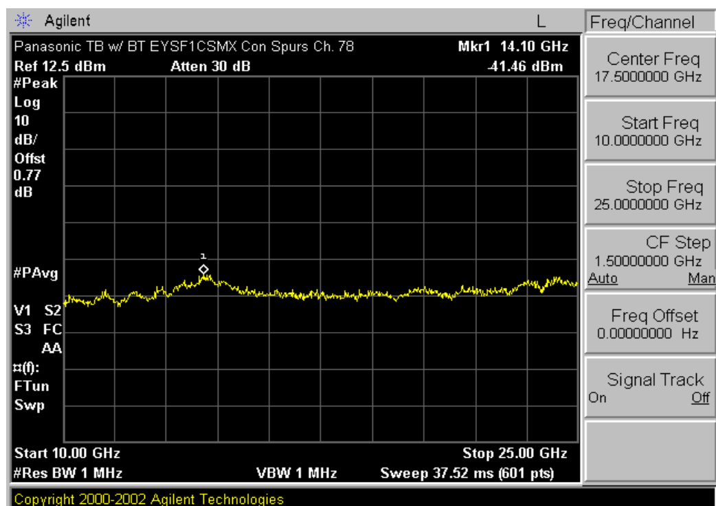
Plot 6-15. Conducted Spurious Plot (Bluetooth – Ch. 78)
