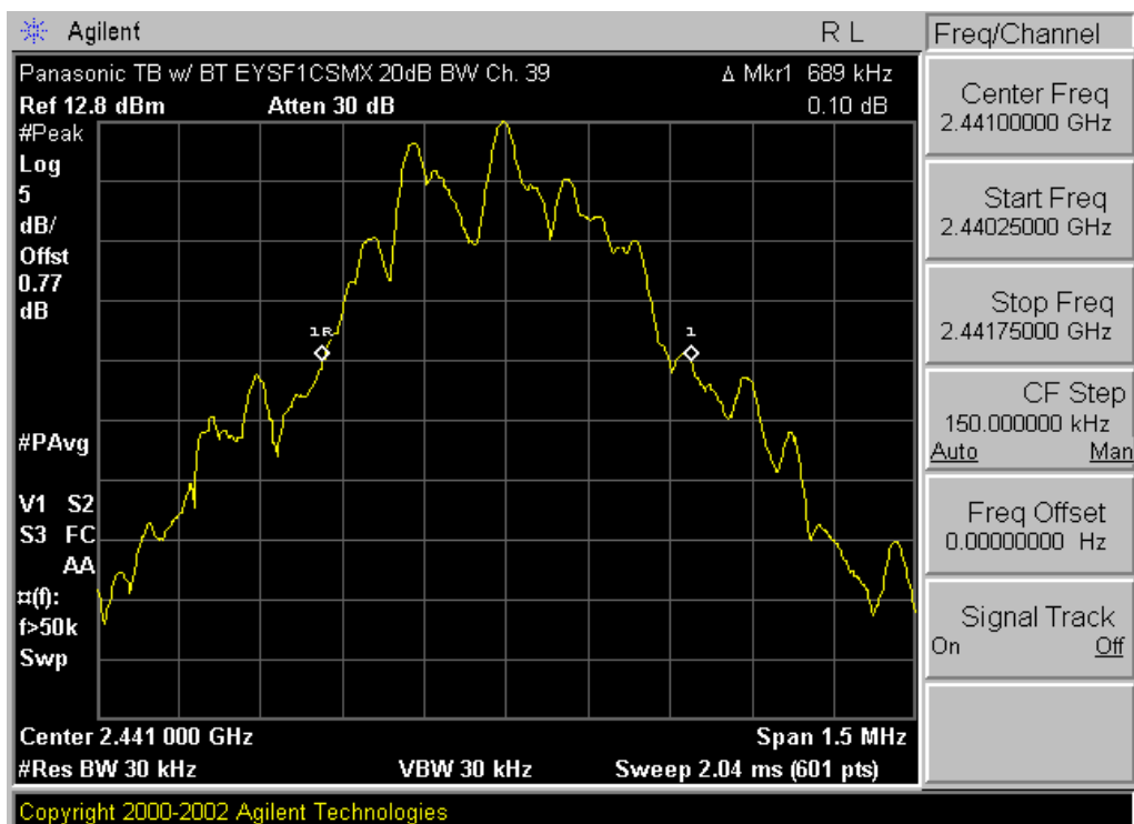
Plot 6-2. 20dB Bandwidth Plot (Bluetooth – Ch. 39)
