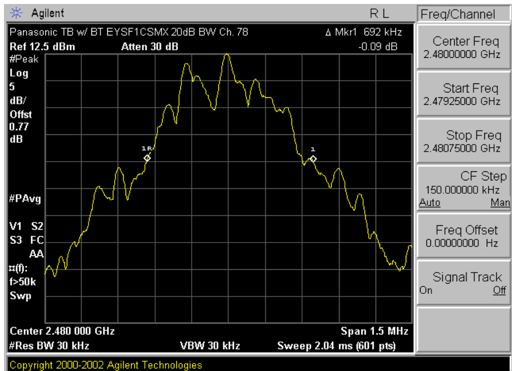
Plot 6-3. 20dB Bandwidth Plot (Bluetooth – Ch. 78)
