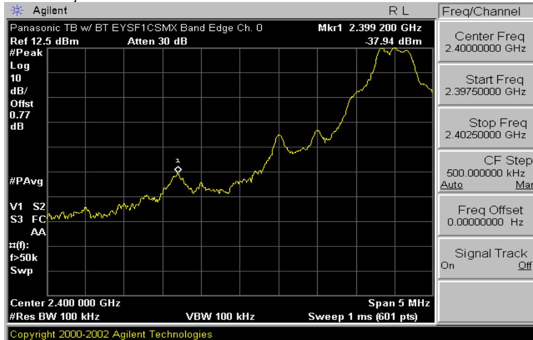
Plot 6-4. Band Edge Plot (Bluetooth – Ch. 0)
