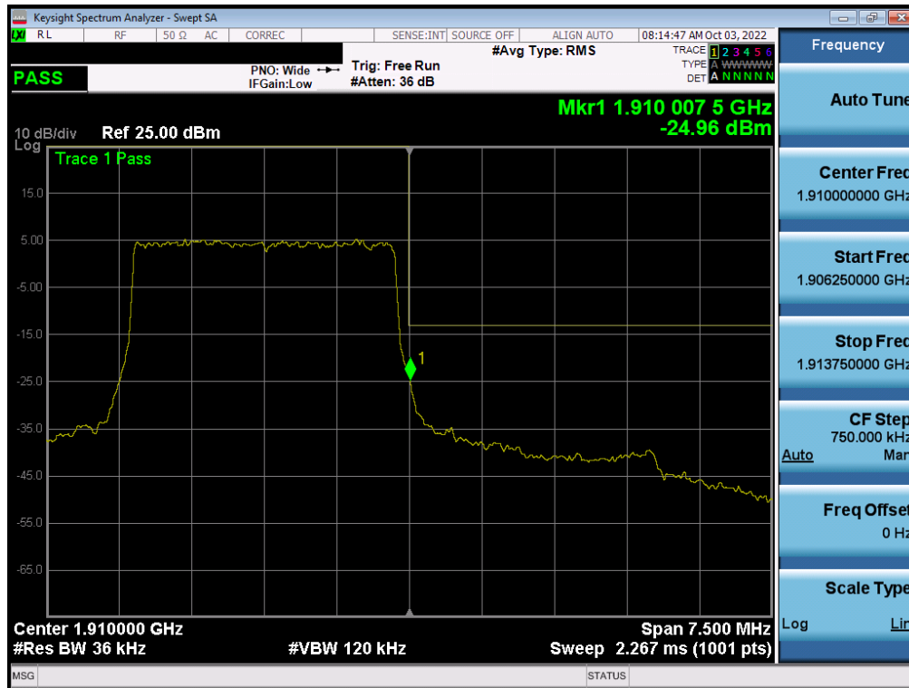
Plot 7-186. Upper Band Edge Plot (LTE Band 2 - 3MHz QPSK – Full RB - ANT F)
