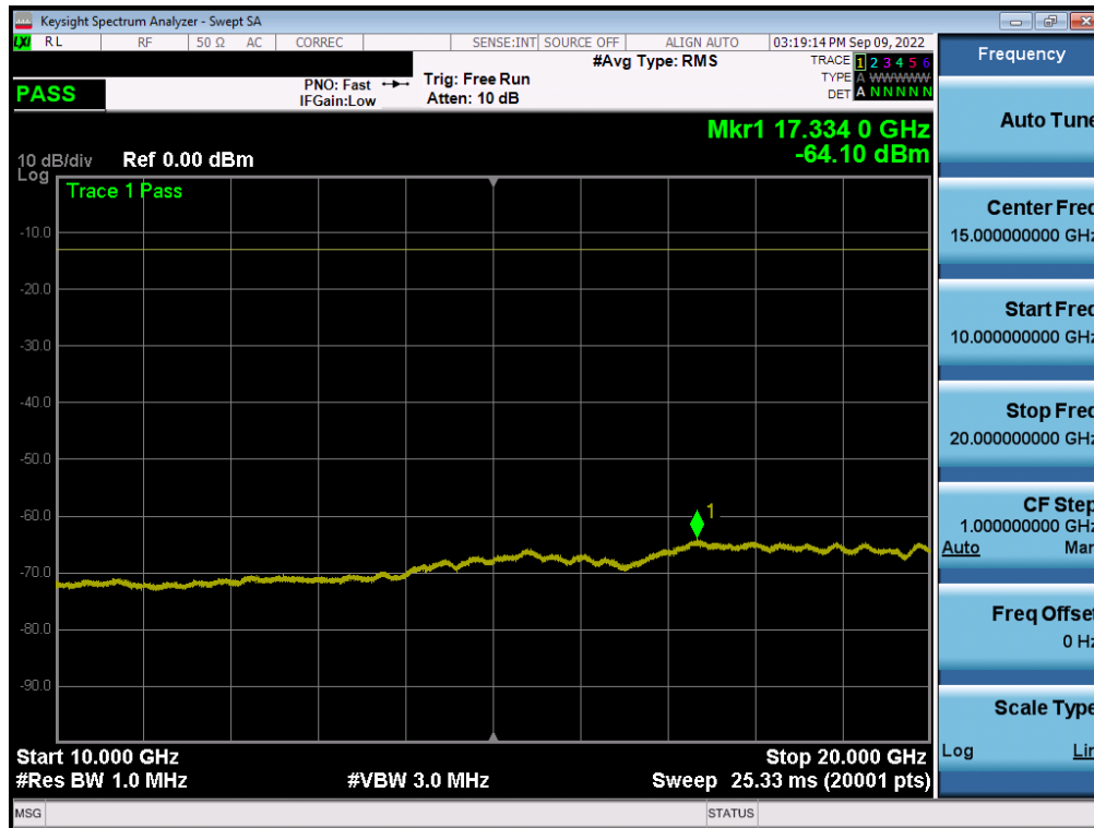
Plot 7-123. Conducted Spurious Plot (WCDMA Ch. 9538 - ANT A)
