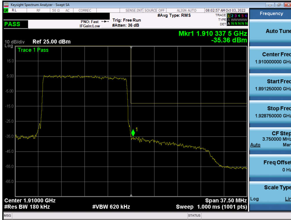
Plot 7-168. Upper Band Edge Plot (LTE Band 2 - 15MHz QPSK – Full RB - ANT F)
