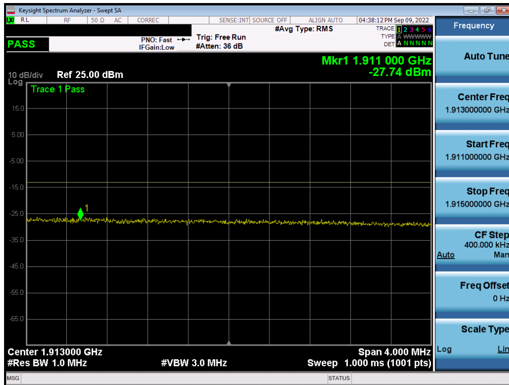
Plot 7-127. Extended Upper Band Edge Plot (LTE Band 2 - 20MHz QPSK – Full RB - ANT A)
