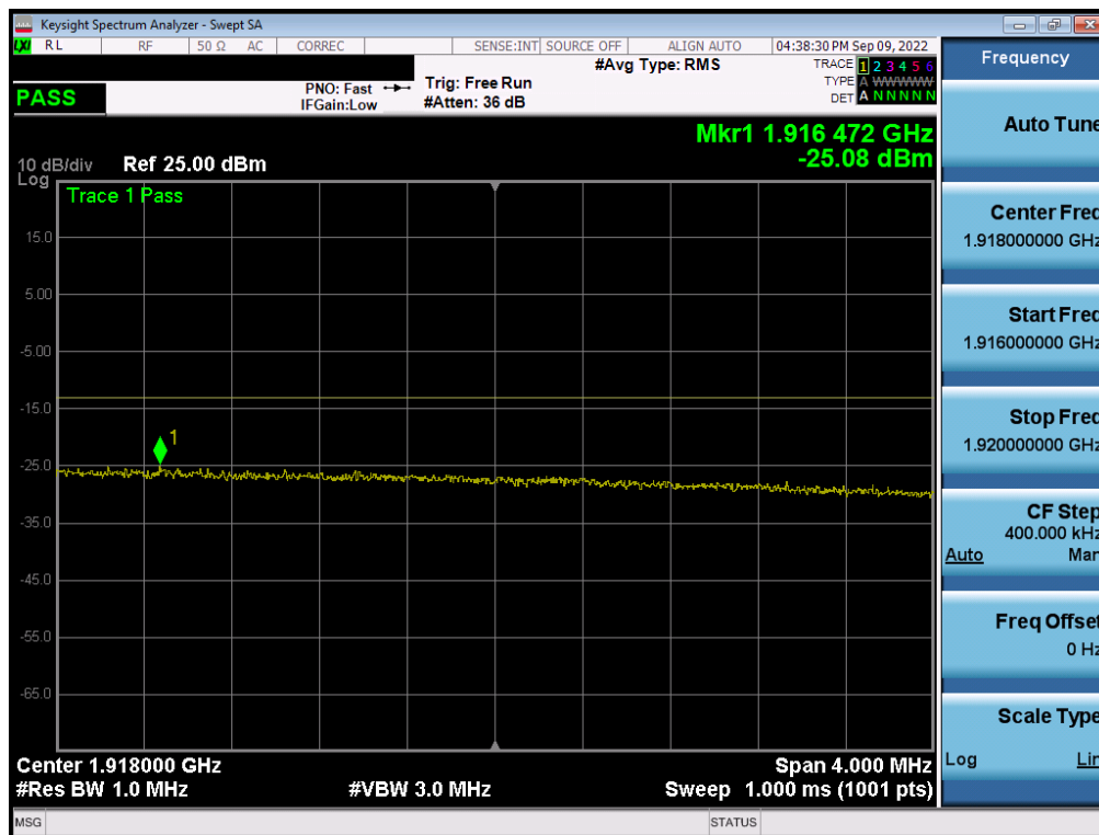
Plot 7-129. Extended Upper Band Edge Plot (LTE Band 25 - 20MHz QPSK – Full RB - ANT A)
