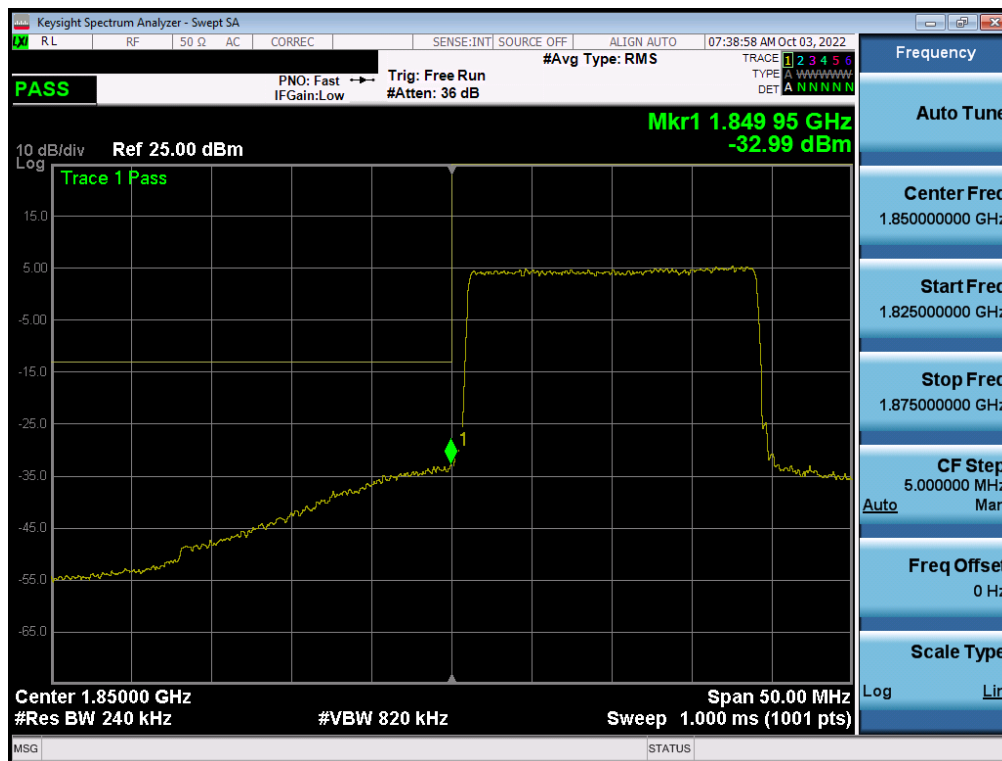
Plot 7-160. Lower Band Edge Plot (LTE Band 25/2 - 20MHz QPSK – Full RB - ANT F)
