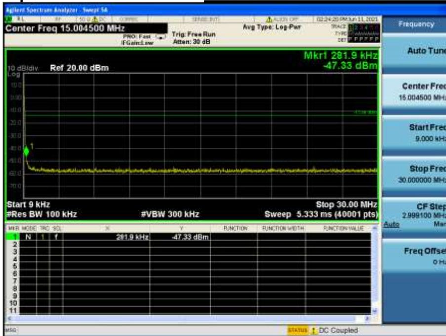
**Conducted Spurious Emissions Middle Channel & Modulation : 8DPSK**
