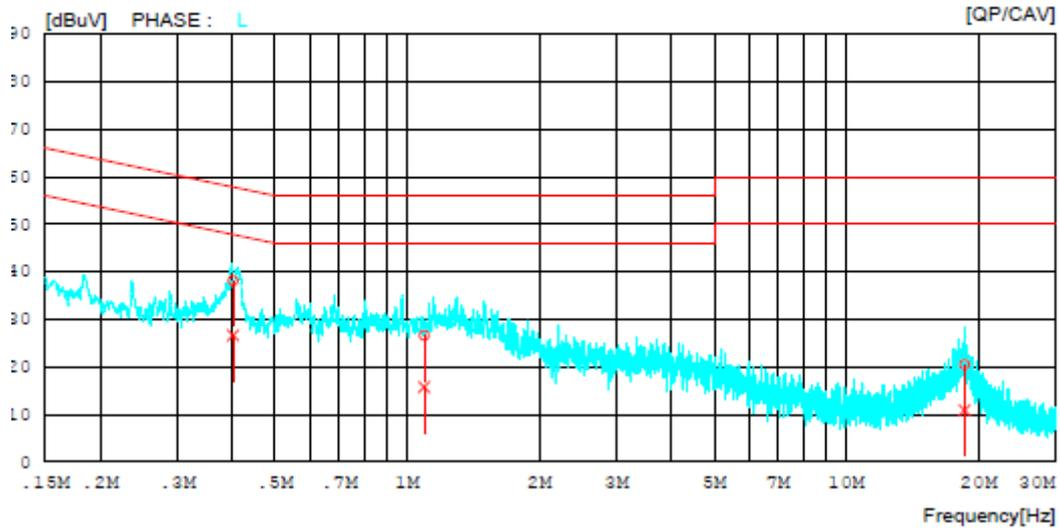
**AC Power-Line Conducted Emissions (List) = Modulation : 8DPSK**
