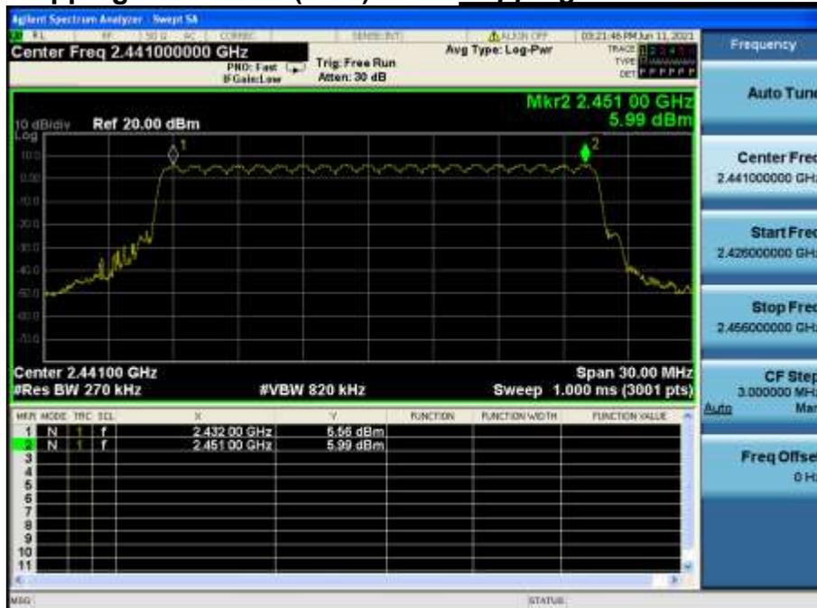
**Number of Hopping Channels 1(AFH)      *Hopping mode : Enable & 8DPSK***
