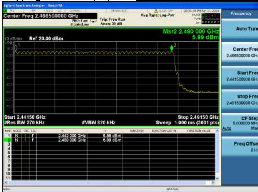
Number of Hopping Channels 1(AFH) Hopping mode : Enable &GFSK
