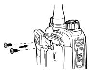
Step 3 Tighten the screws.
