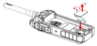
Step 2 Replace the cover and tighten the screw as shown below.
