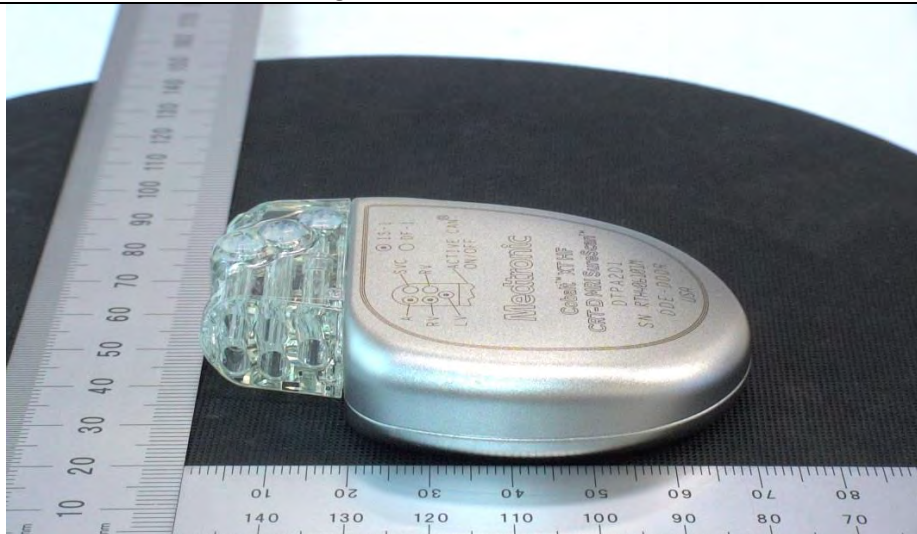
Model Cobalt XT HF CRT-D MRI SureScan – left angle
