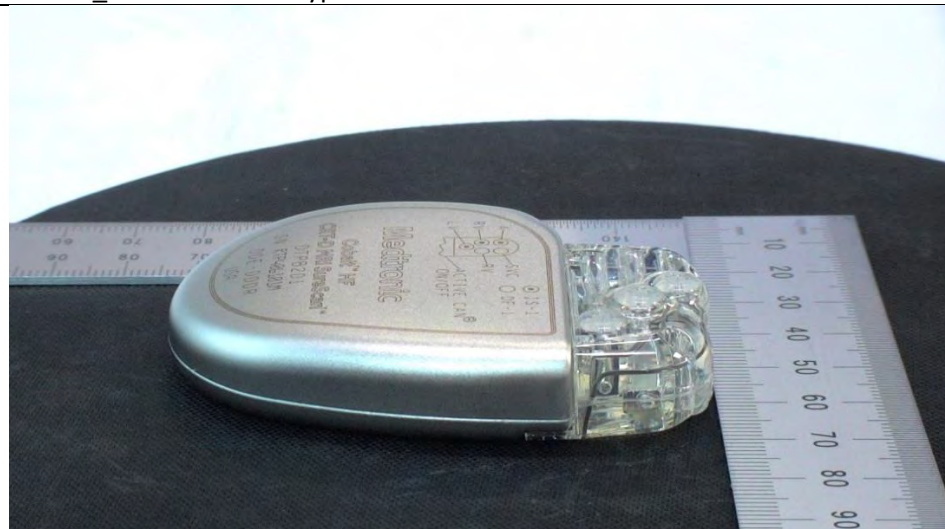
Model Cobalt HF CRT-D MRI SureScan – right angle
