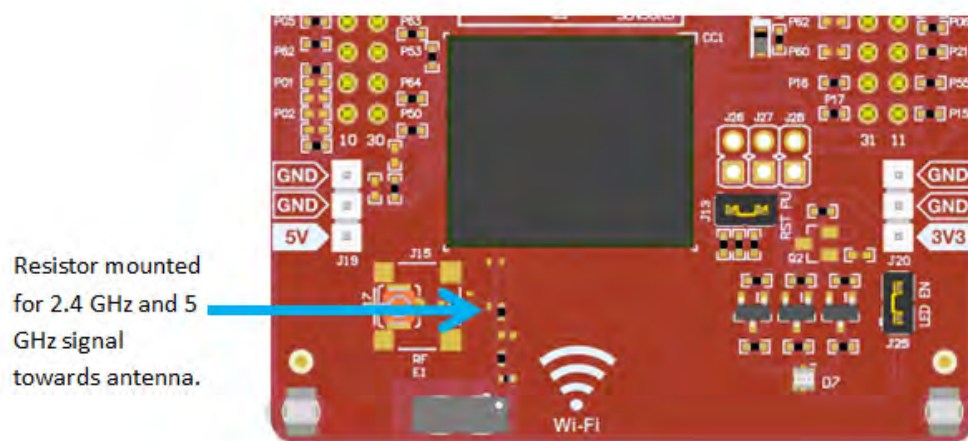
Figure 28. Using Onboard Antenna (Default Condition)
