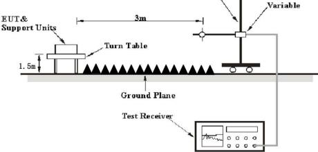
The radiated emission tests were performed in the 3 meters, using the setup accordance with the ANSI C63.10-2013. The specification used was the FCC 15.209 and FCC 15.247 limits.
