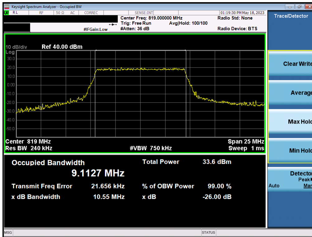
Plot 7-7. Occupied Bandwidth Plot (LTE Band 26 - 10MHz QPSK - Full RB Configuration)
