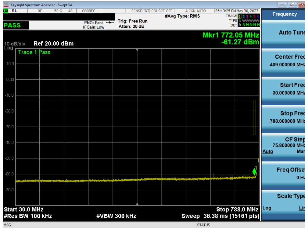
Plot 7-26. Conducted Spurious Plot (LTE Band 14 - 5MHz QPSK - RB Size 1, RB Offset 0 - High Channel)
