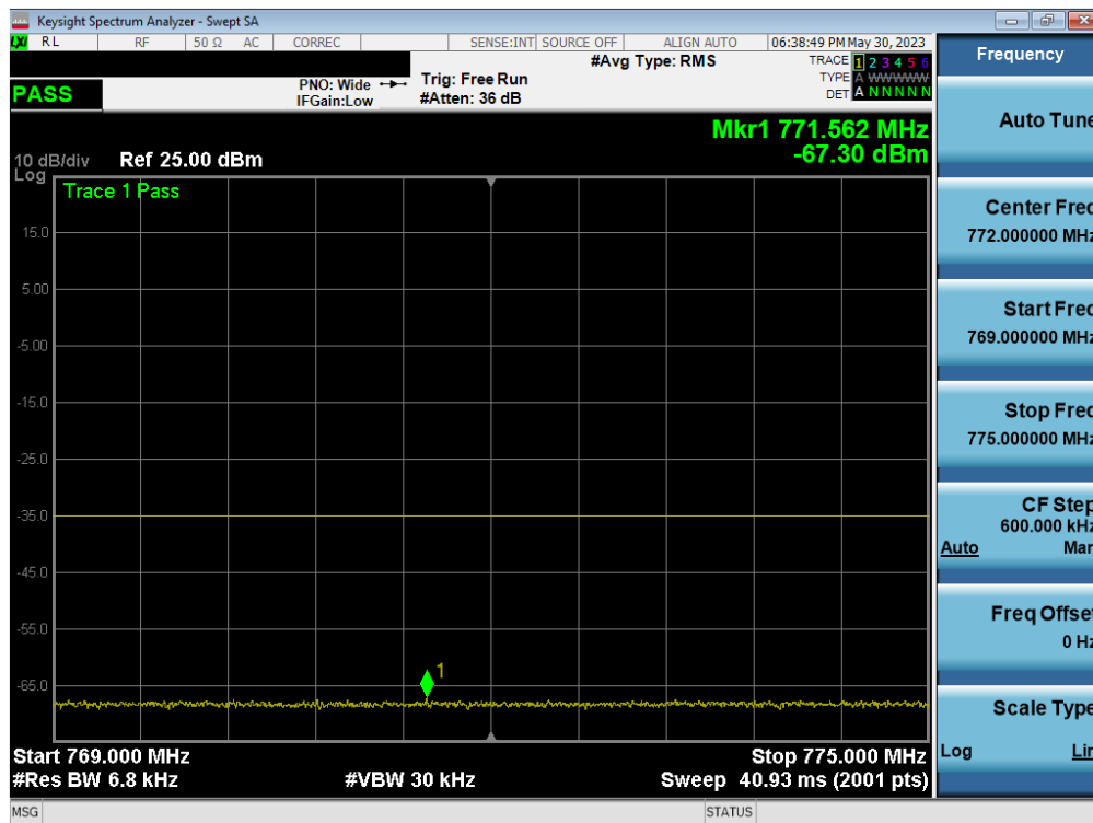
Plot 7-39. Lower Emission Mask Plot (LTE Band 14, 5MHz QPSK - RB Size 25)
