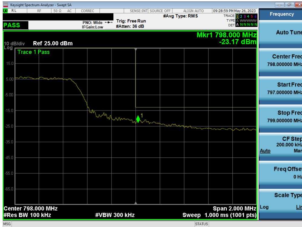
Plot 7-44. Upper Band Edge Plot (LTE Band 14, 10MHz QPSK - RB Size 50)
