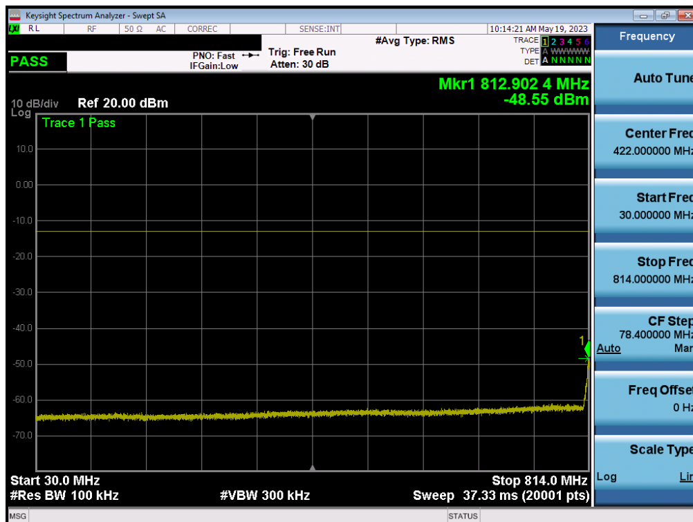
Plot 7-19. Conducted Spurious Plot (LTE Band 26 - 5MHz QPSK - RB Size 1, RB Offset 0 – High Channel)
