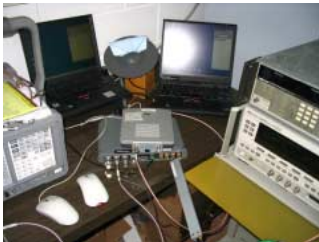
Photograph 7.3.1 Peak spectral power density test setup
