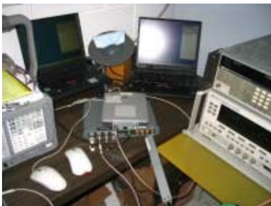
Photograph 7.1.1 The 6 dB bandwidth test setup
