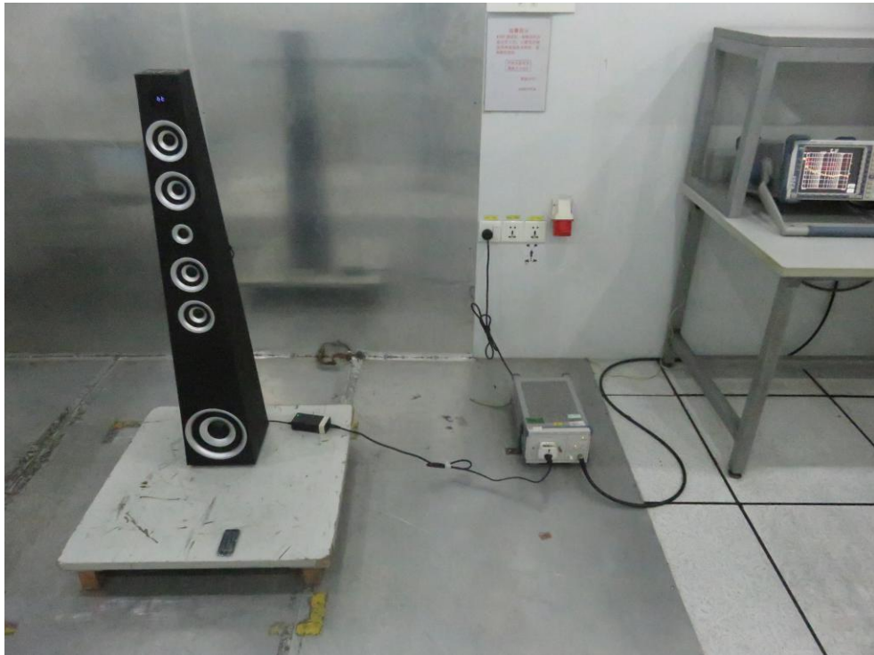
Photo of Conducted Emission Measurement
