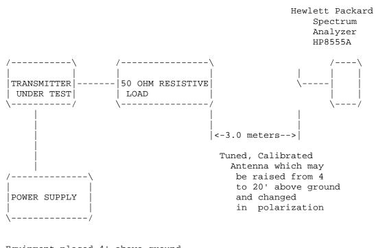
Equipment placed 4' above ground on a rotatable platform.
