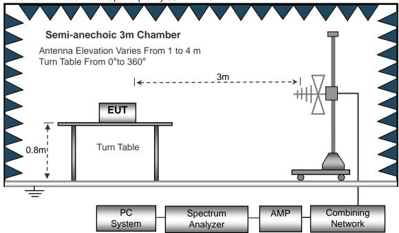
(C) Radiated Emission Test-Up Frequency Above 1GHz
