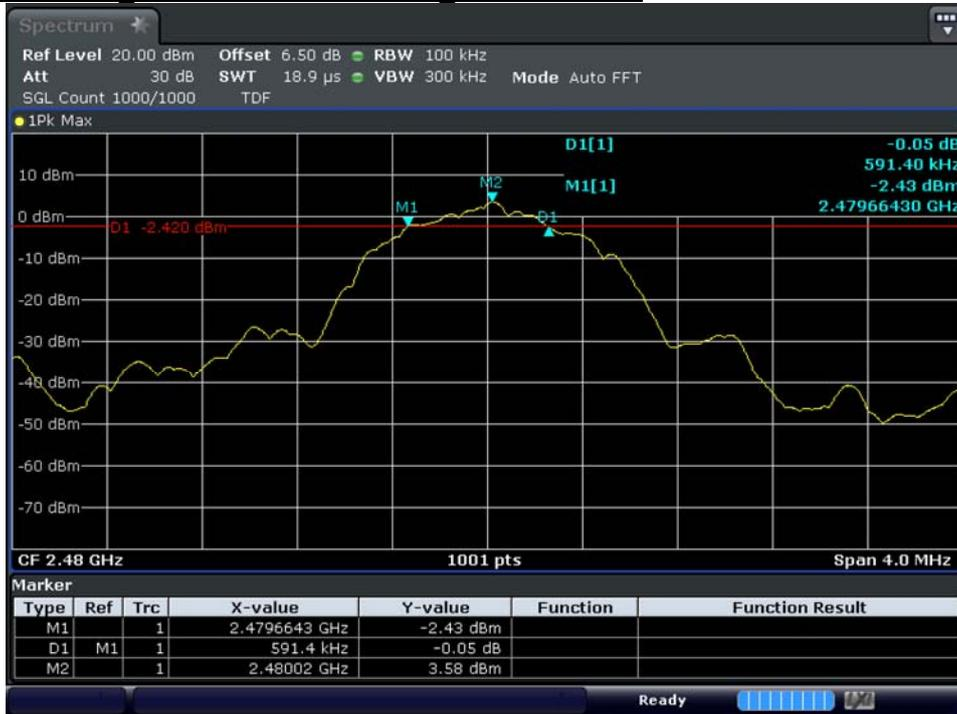
Test mode : SLAVE Bluetooth LE / 2 402 MHz Occupied Bandwidth
