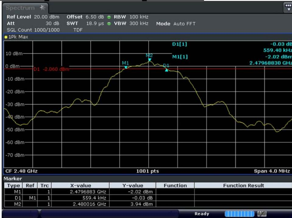
Test mode : MASTER Bluetooth LE / 2 402 MHz Occupied Bandwidth
