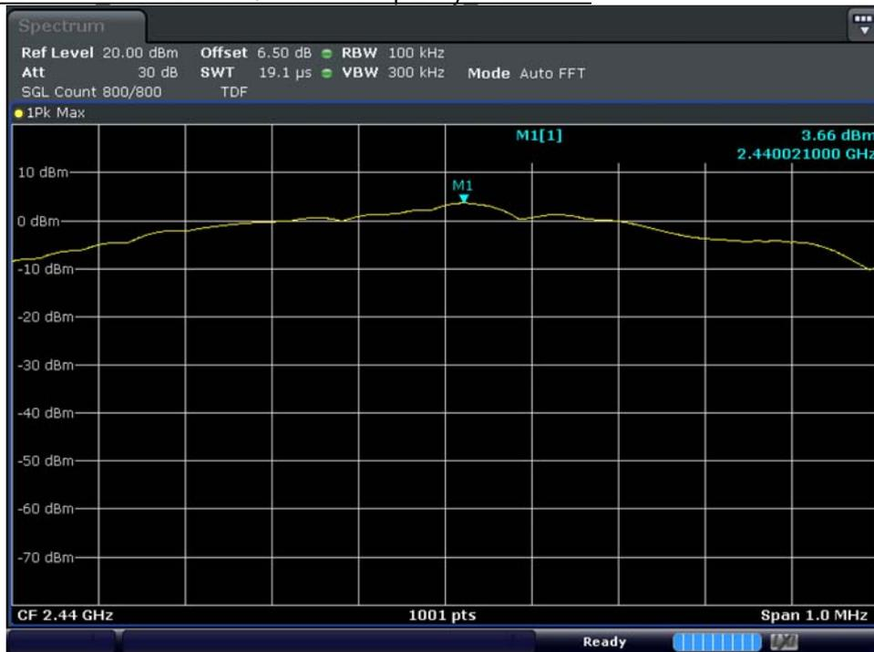
Test mode : SLAVE Bluetooth LE / Middle Frequency Conducted Spurious Emission
