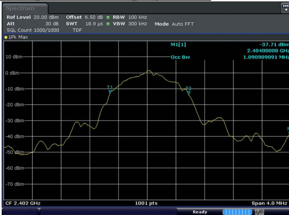
Test mode : SLAVE Bluetooth LE / 2 440 MHz Occupied Bandwidth
