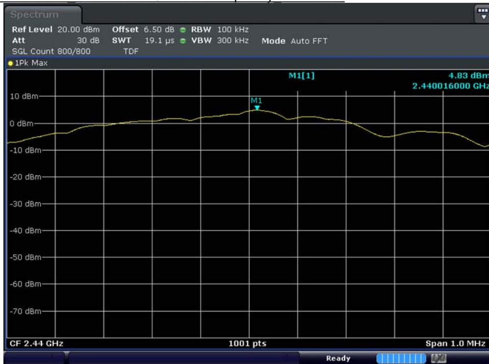
Test mode : MASTER Bluetooth LE / Middle Frequency Conducted Spurious Emission
