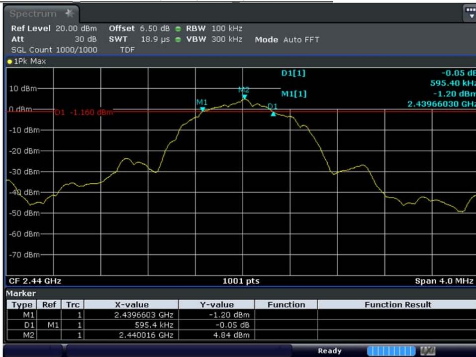
Test mode : MASTER Bluetooth LE / 2 480 MHz 6 dB Bandwidth
