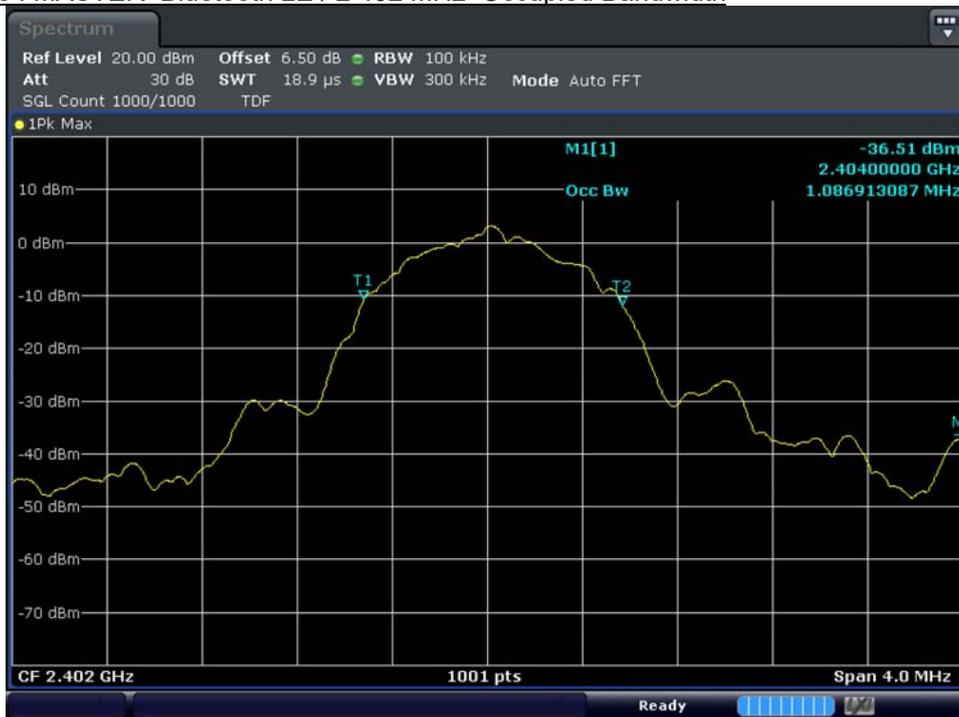
Test mode : MASTER Bluetooth LE / 2 440 MHz Occupied Bandwidth
