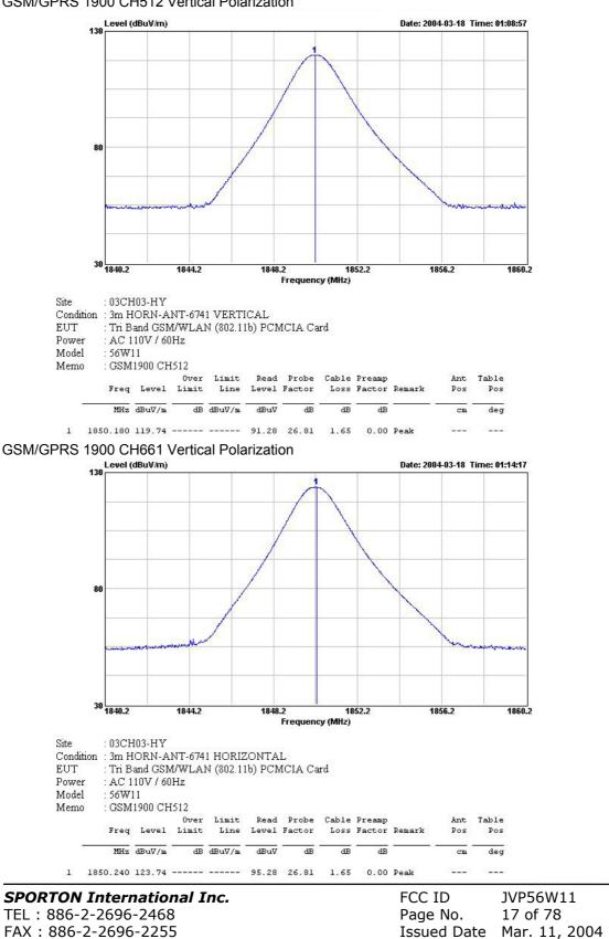
GSM/GPRS 1900 CH512 Vertical Polarization
