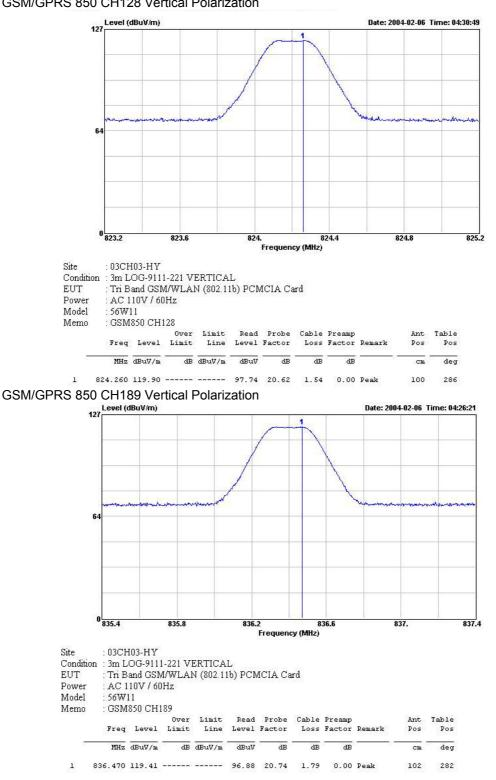
GSM/GPRS 850 CH128 Vertical Polarization
