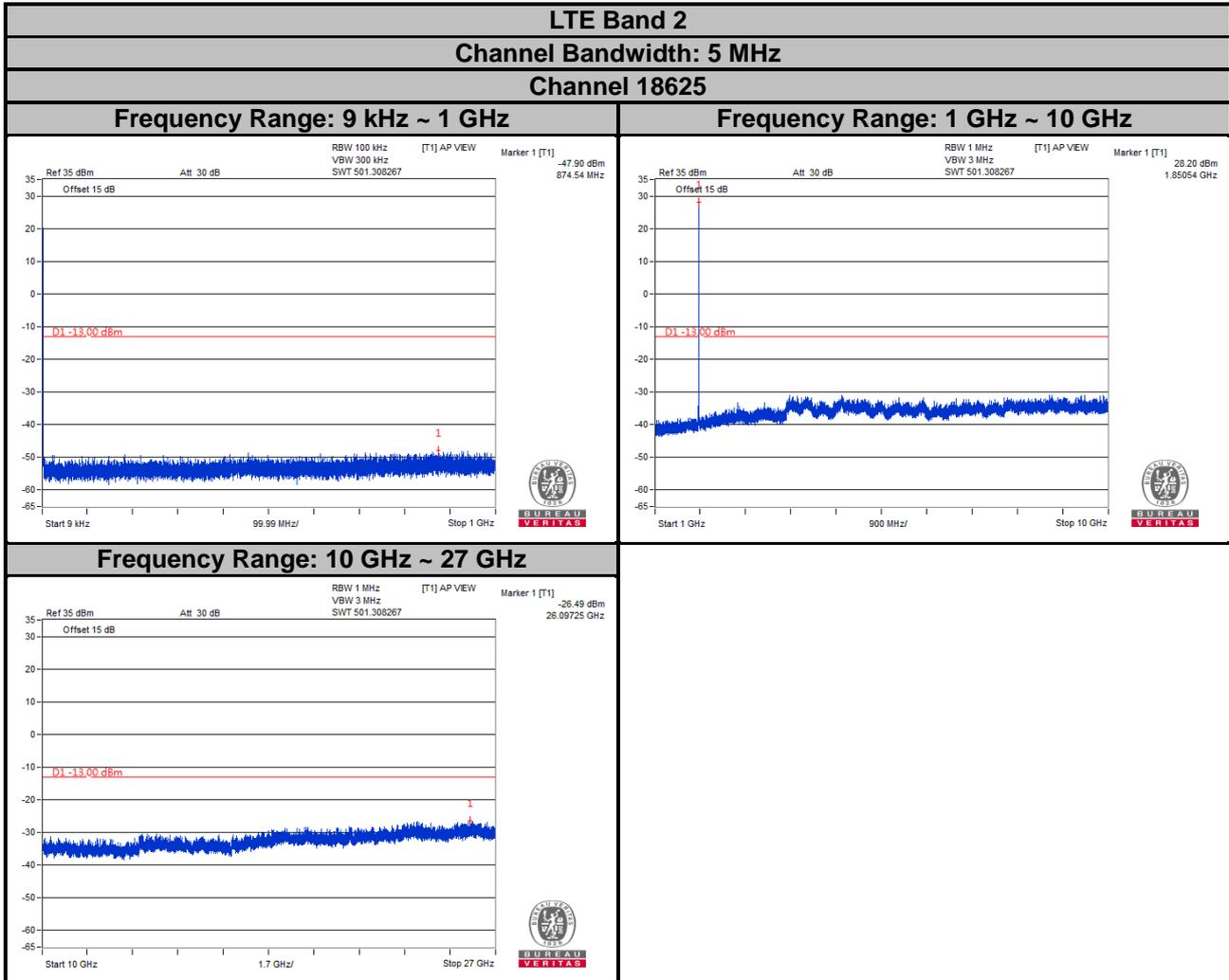
Note: The signal over the limit in 9 kHz is from spectrum analyzer.
