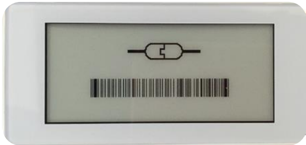
Connected to gateway
