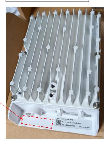
In compliance with 47 CFR 2.925(d)(1), the label is permanently affixed to the equipment by means of a permanent adhesive coating the back of a printed label at the location identified in the product photo shown.
