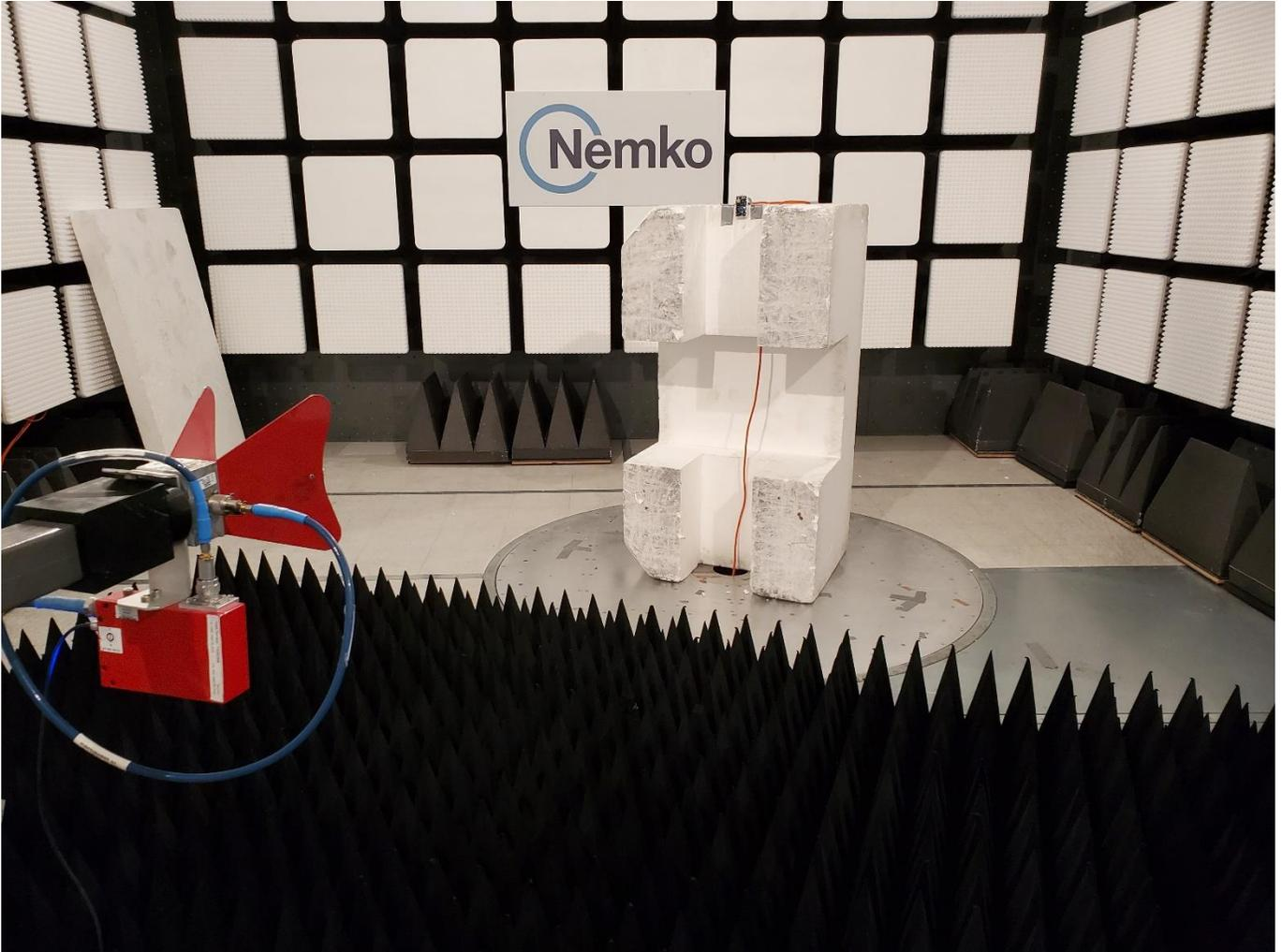
1.4 Radiated emissions above 1 GHz, Rear view
