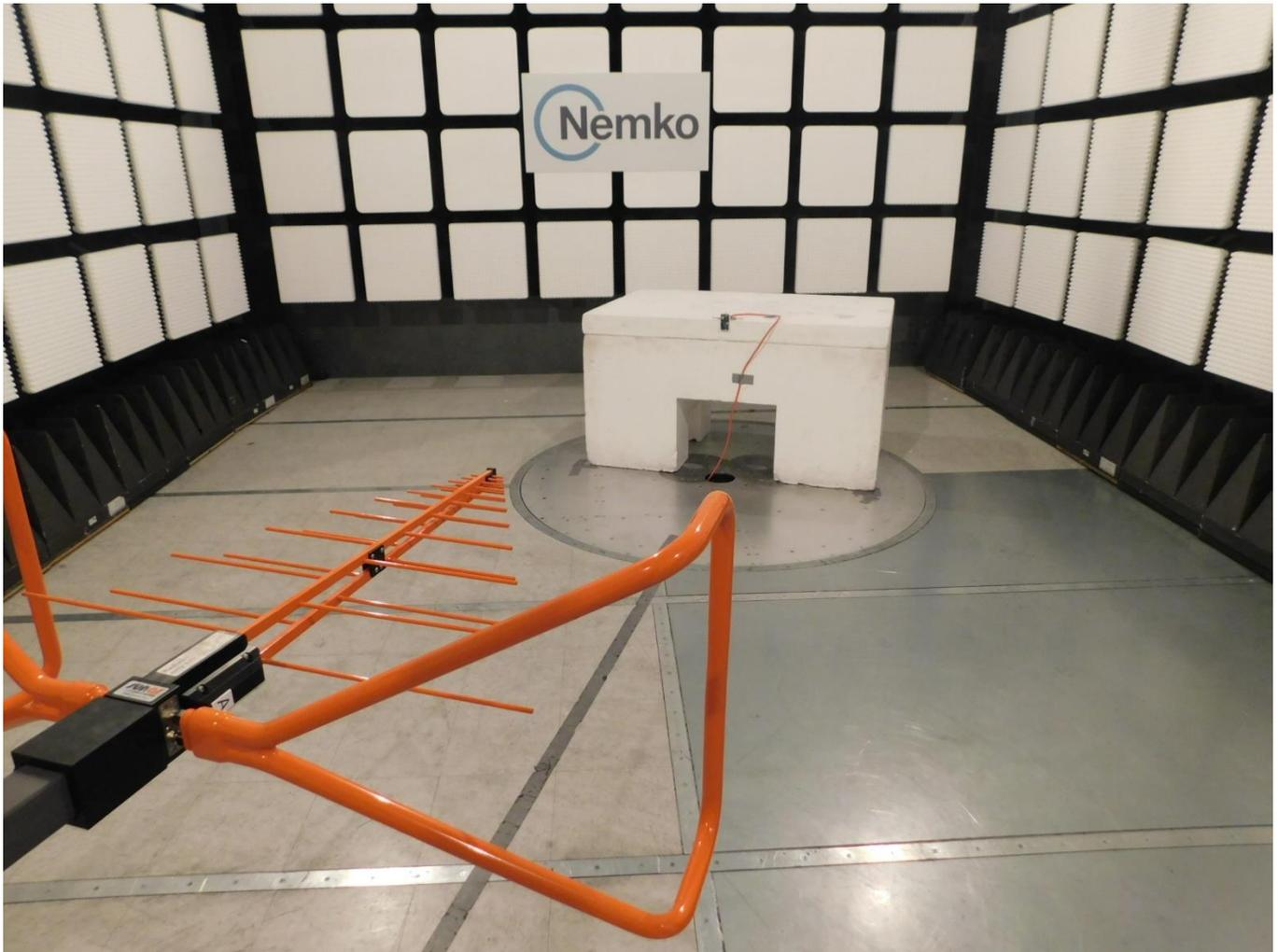
1.2 Radiated emissions below 1 GHz, Rear view
