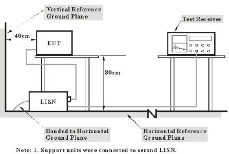
Note: 1. Support units were connected to second LISN. 2. Both of LISNs (AMIN) 80 cm from EUT and at the least 80 cm from other units and other metal planes support units.
