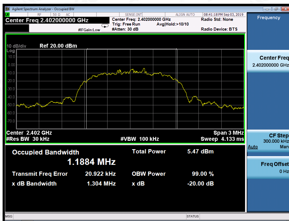
TEST PLOT OF BANDWIDTH FOR LOW CHANNEL
