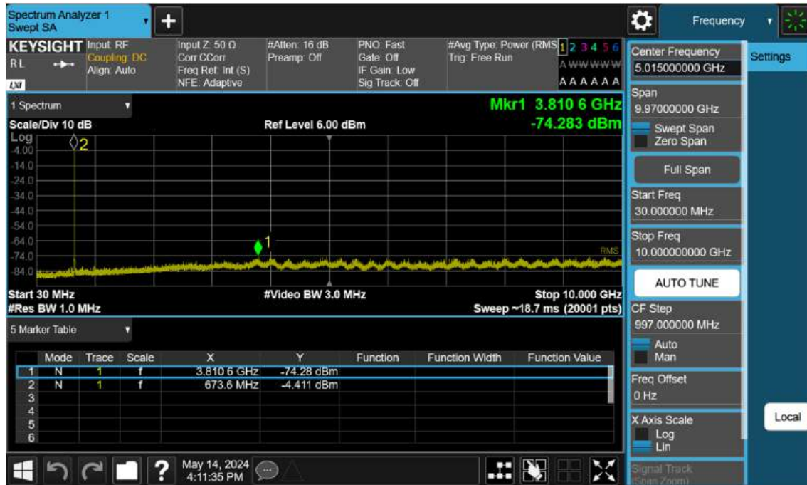
Sub6 n71. Conducted Spurious Plot _ (136100ch_15 MHz_BPSK_RB 1_1)
