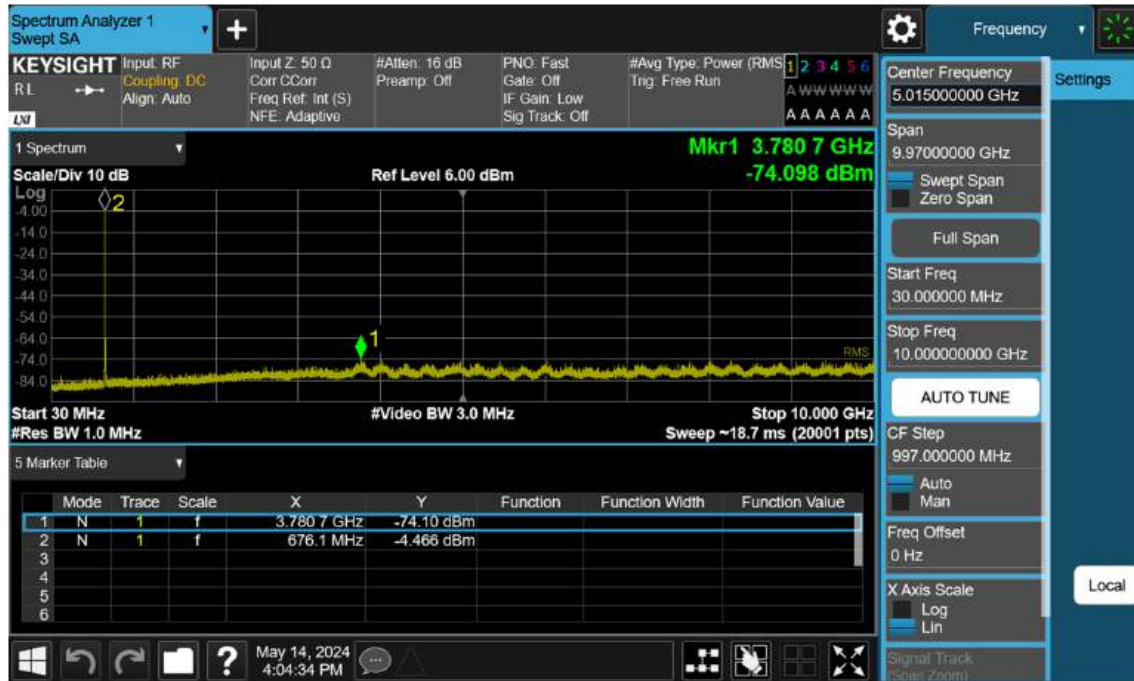
Sub6 n71. Conducted Spurious Plot _ (136100ch_10 MHz_BPSK_RB 1_1)
