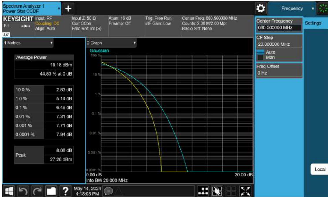
Sub6 n71. PAR Plot (20 M BW_Ch.349000_256 QAM_Full RB)
