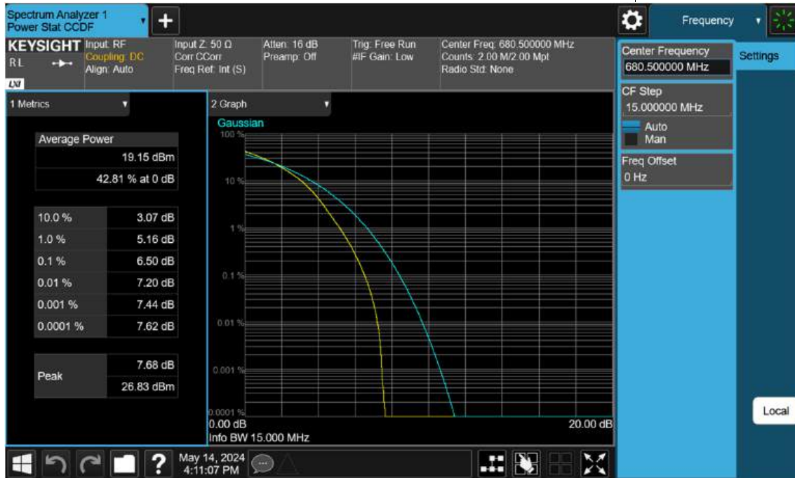
Sub6 n71. PAR Plot (15 M BW_Ch.349000_256 QAM_Full RB)
