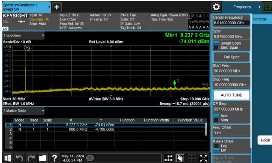
Sub6 n71. Conducted Spurious Plot _ (138600ch_10 MHz_BPSK_RB 1_1)
