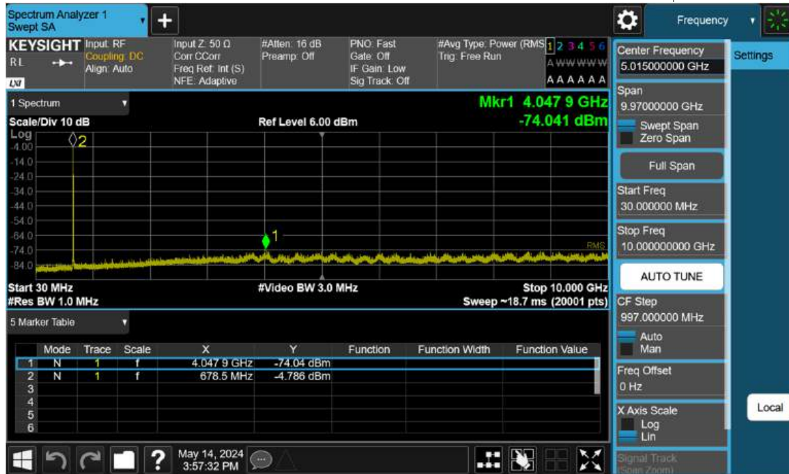
Sub6 n71. Conducted Spurious Plot _ (136100ch_5 MHz_BPSK_RB 1_1)
