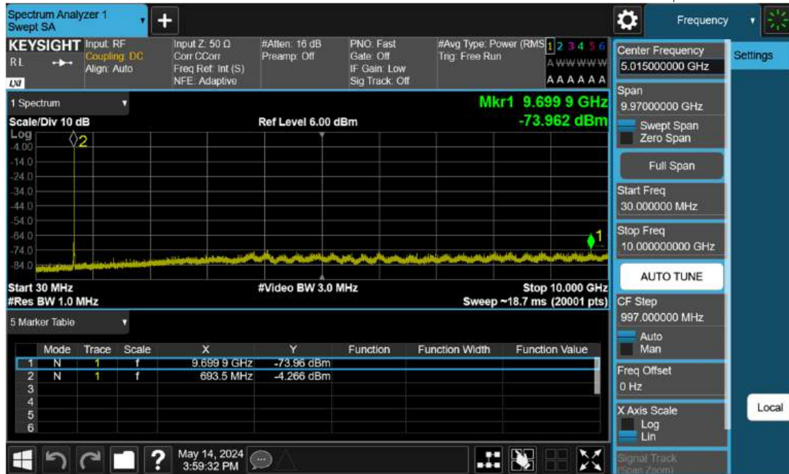
Sub6 n71. Conducted Spurious Plot _ (139100ch_5 MHz_BPSK_RB 1_1)
