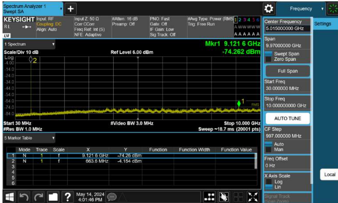
Sub6 n71. Conducted Spurious Plot _ (133600ch_10 MHz_BPSK_RB 1_1)
