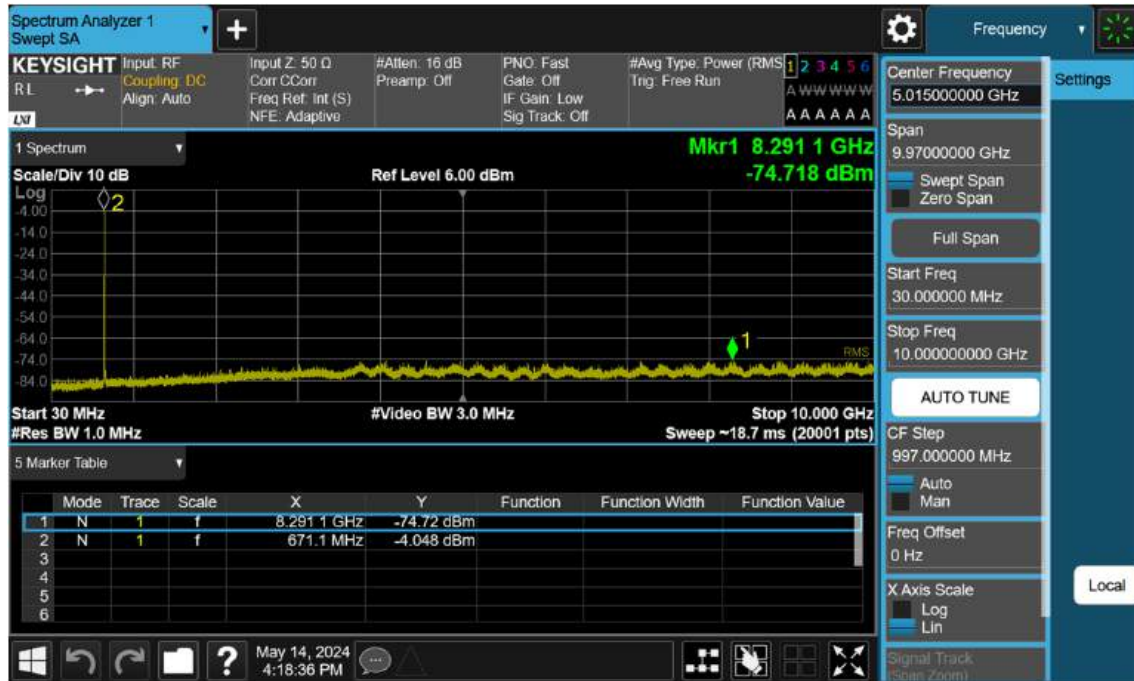
Sub6 n71. Conducted Spurious Plot _ (136100ch_20 MHz_BPSK_RB 1_1)
