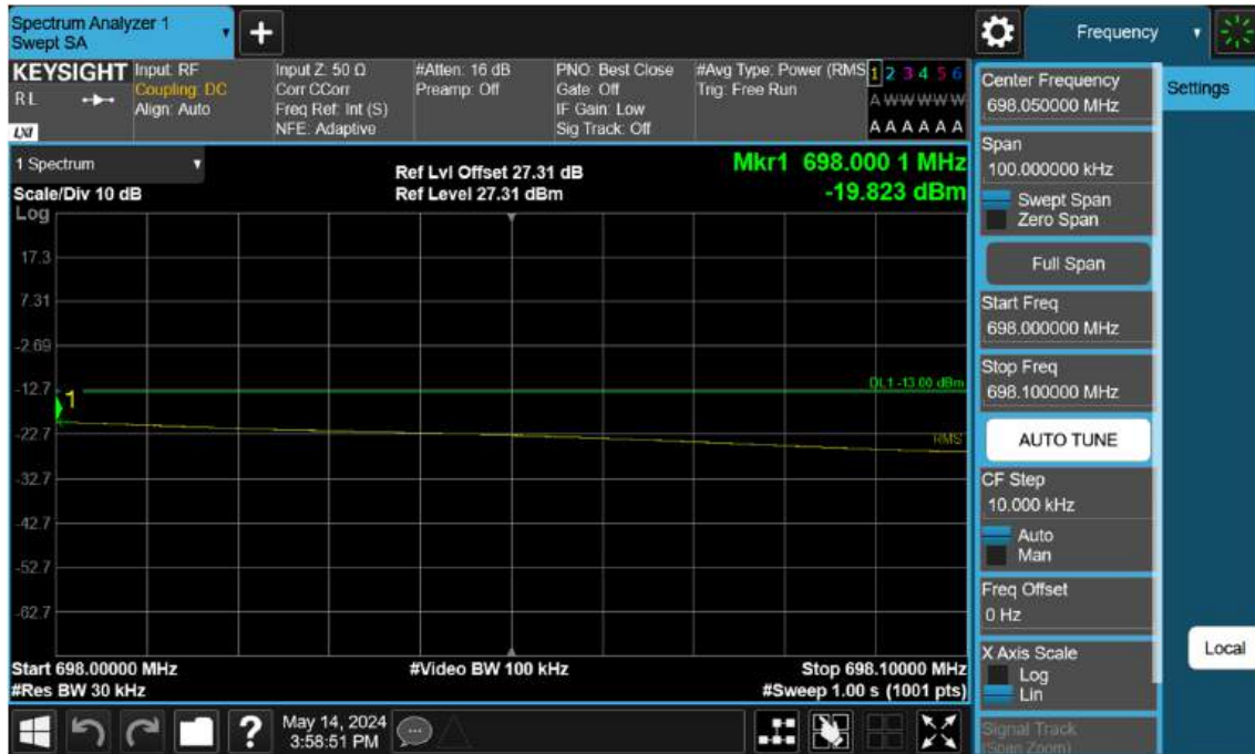
Sub6 n71. Upper Band Edge Plot (5 M BW Ch.139100 BPSK_RB1_Offset 24)_1
