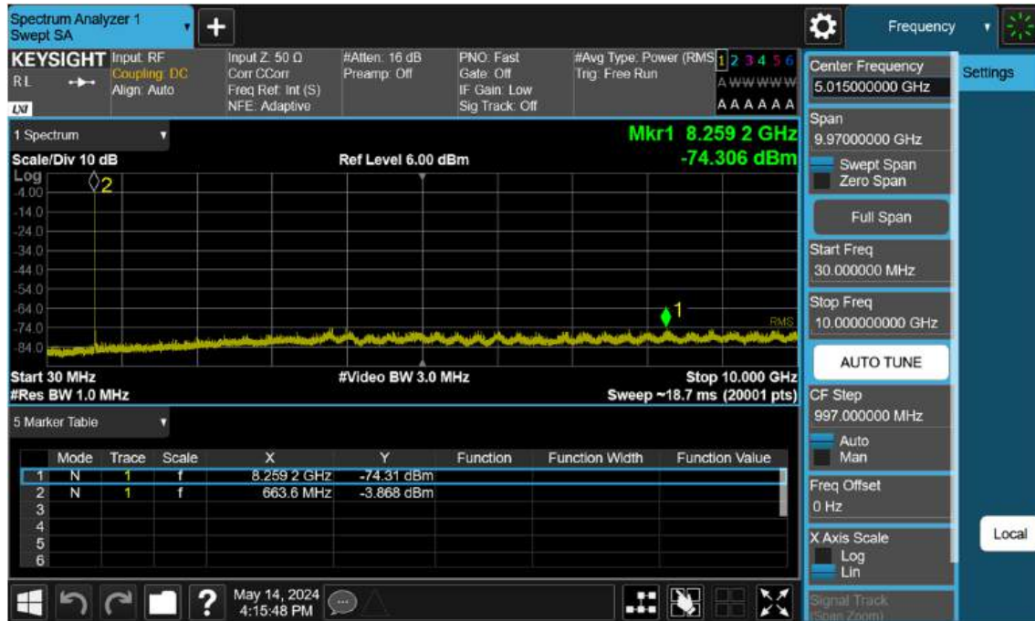
Sub6 n71. Conducted Spurious Plot _ (134600ch_20 MHz_BPSK_RB 1_1)
