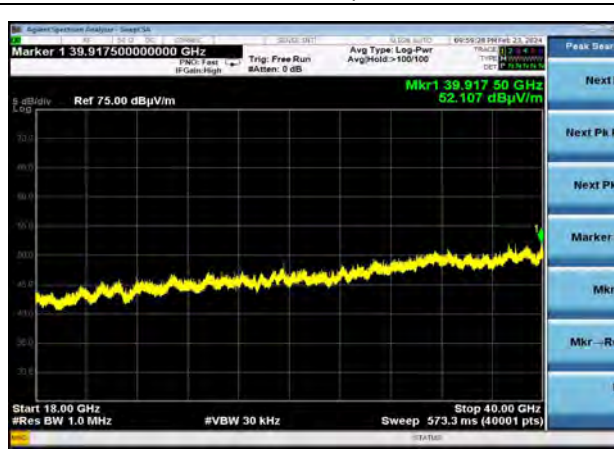
802.11b | Channel 6 | 1 Mbps 18000-40000 MHz | Vertical
