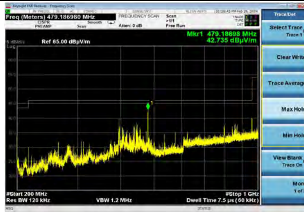
802.11b | Channel 6 | 1 Mbps | 200-1000 MHz | Vertical
