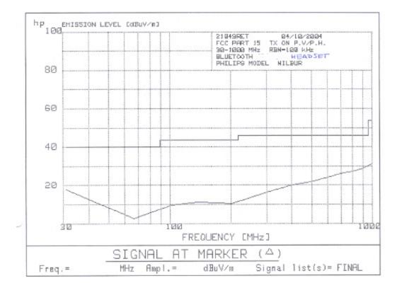
Resolution bandwidth = 100 kHz. Video bandwidth = 100 kHz.
