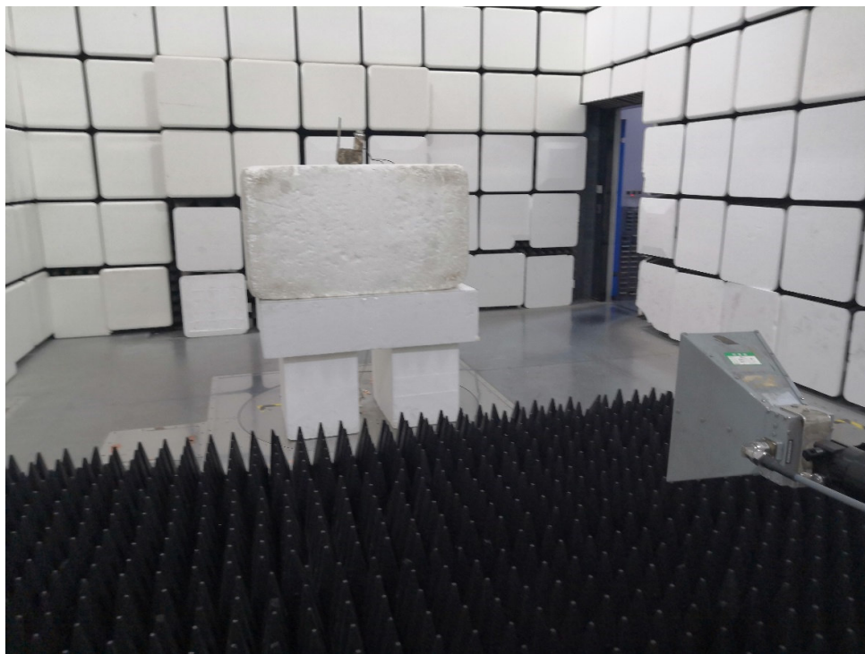
Picture 1 Radiated Spurious Emissions Test setup
