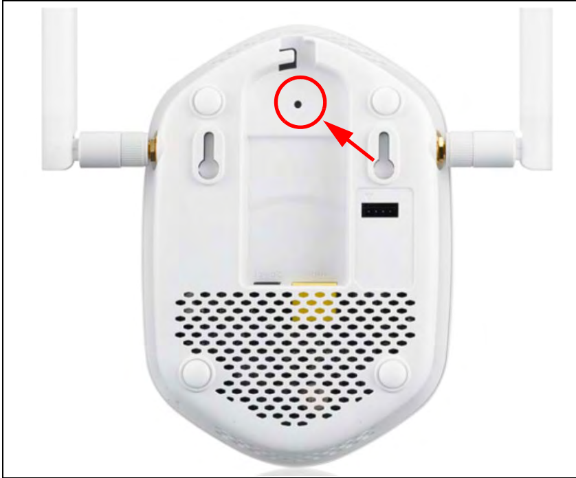
Figure 9 The RESET Button
